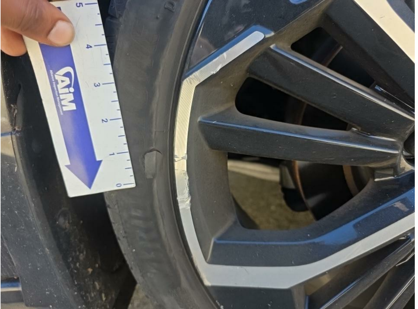
RF Tire Torn Replacement Required
