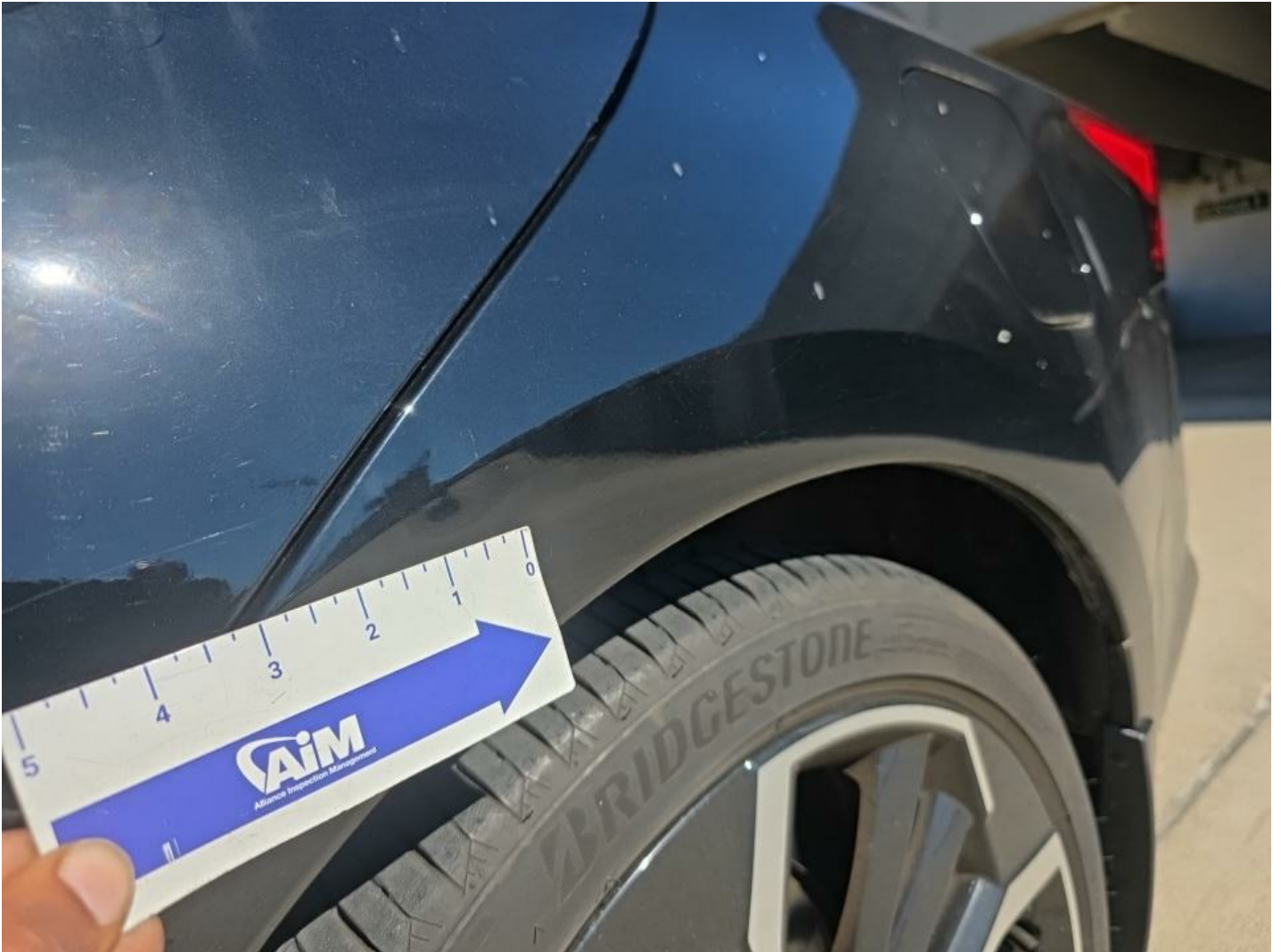
L Qtr Panel Dent/No Paint Dmg 1" to 2"
