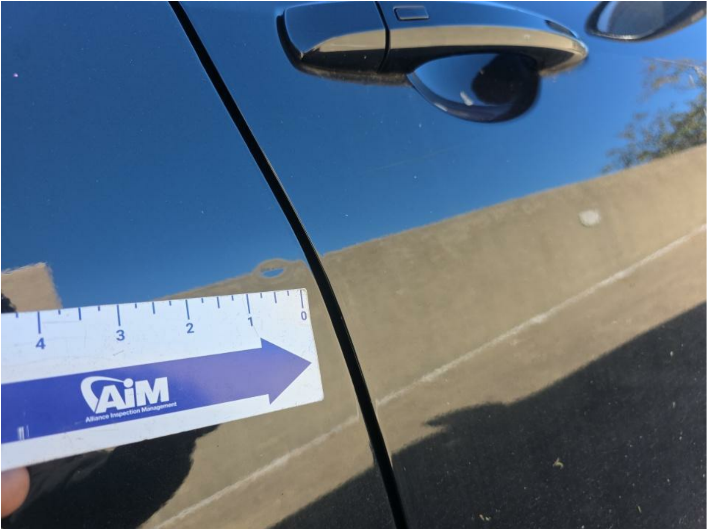
RR Door Dent/No Paint Dmg 1/2" to 1"
