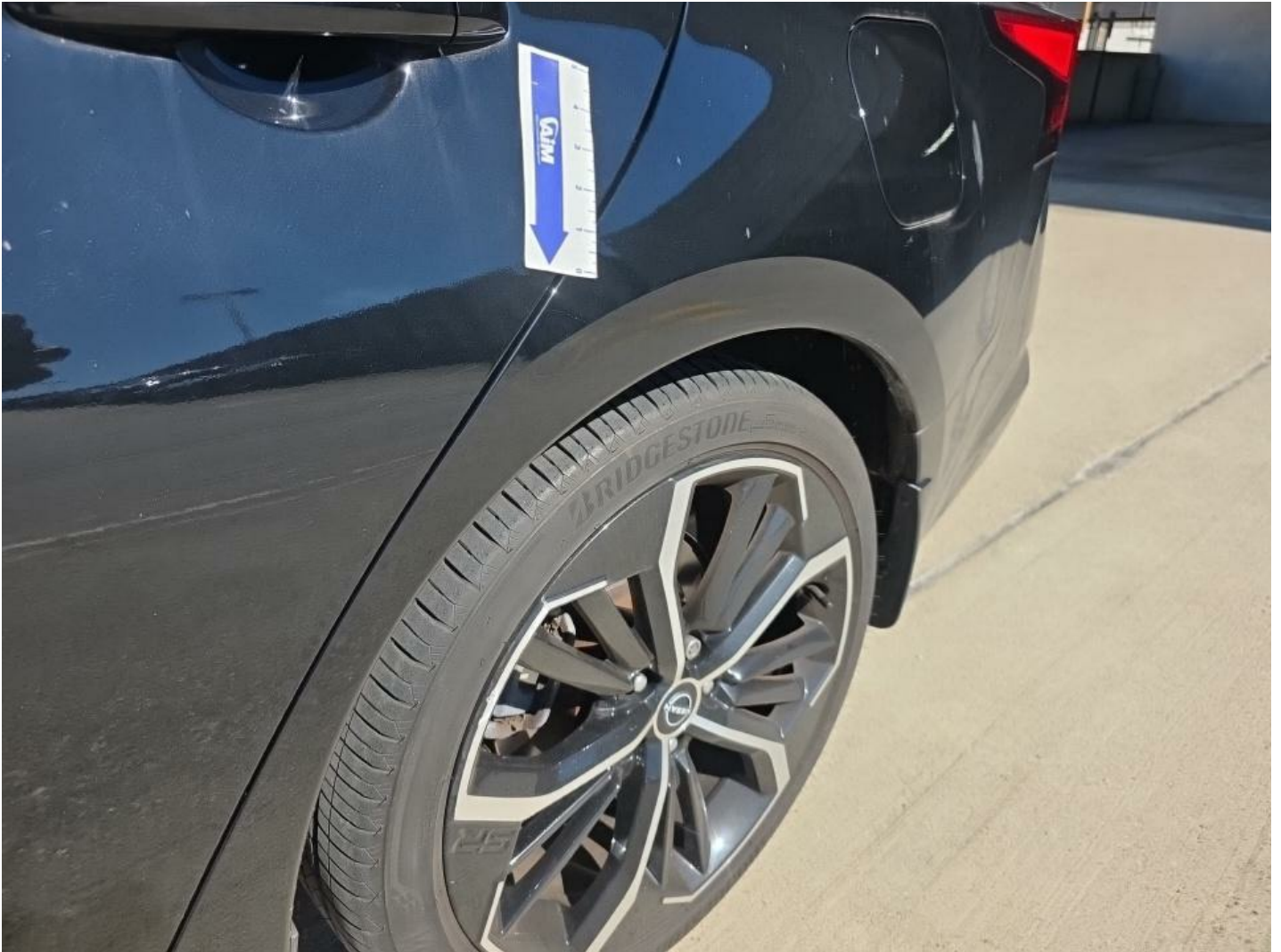
L Qtr Panel Dent/No Paint Dmg 1" to 2"
