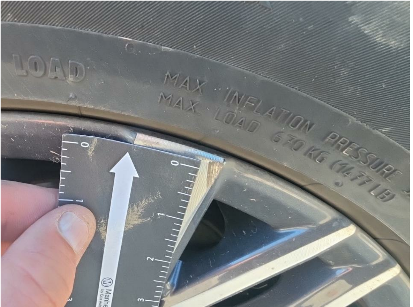
RF Wheel Curb Rash < 1/8"
