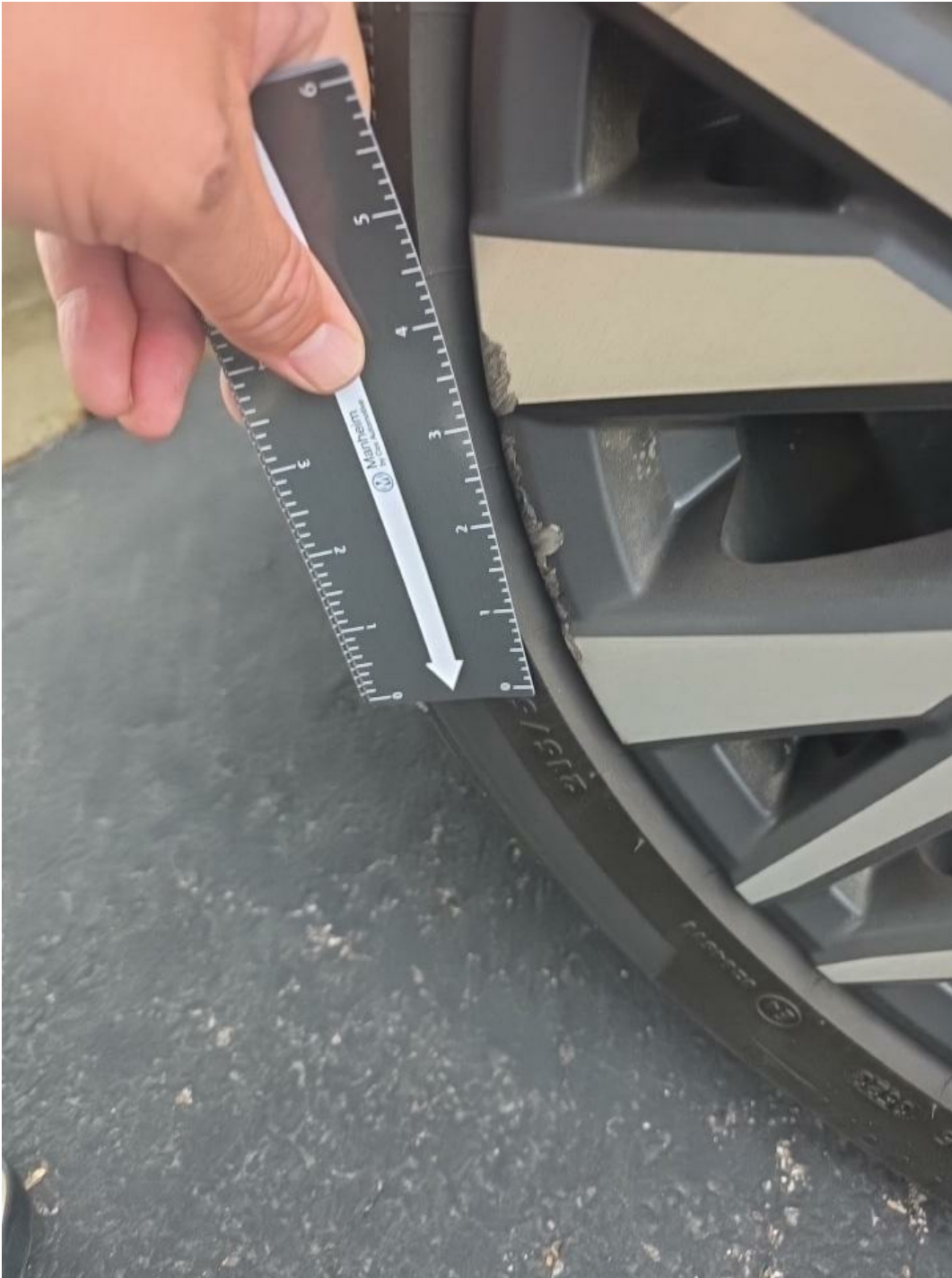
RR Wheel Curb Rash 3" to 4"
