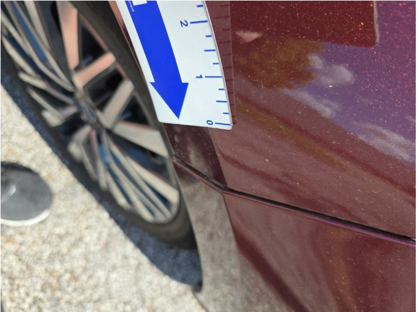
Front Bumper Misaligned Repair Required
