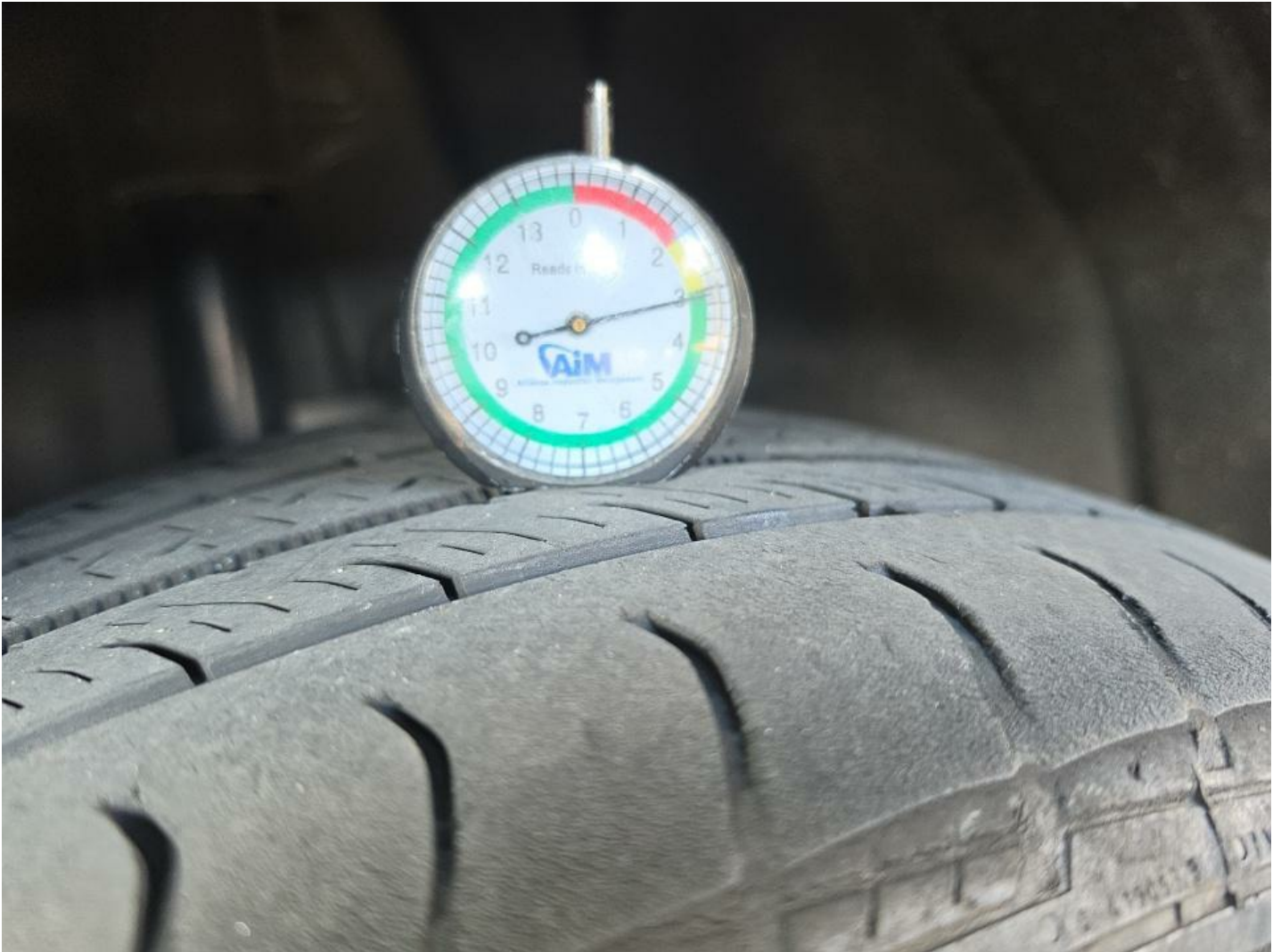
RR Tire Worn Replacement Required
