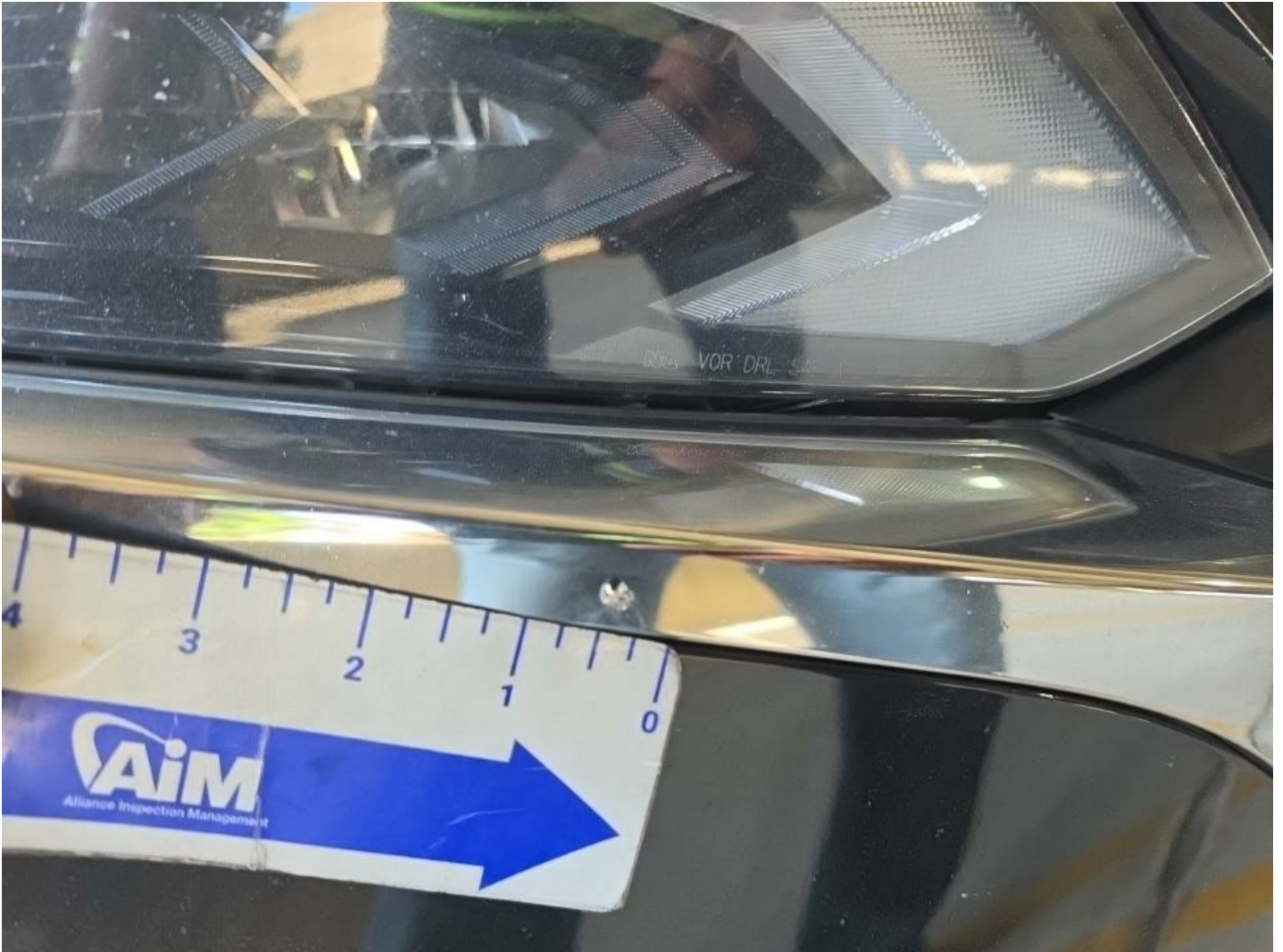
F Bumper Right Molding Chipped 1
