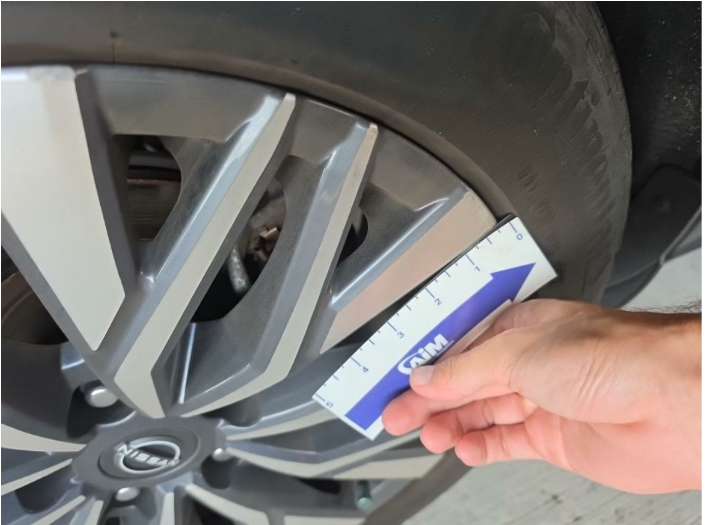
RR Wheel Curb Rash 3" to 4"
