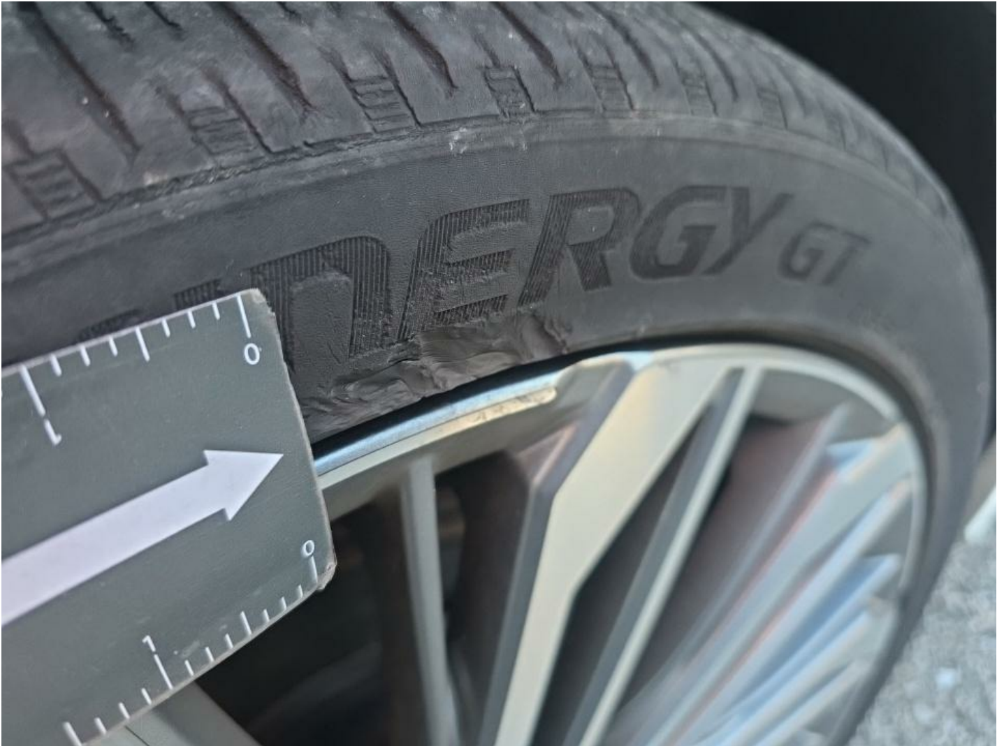
RF Tire Gouged Replacement Required
