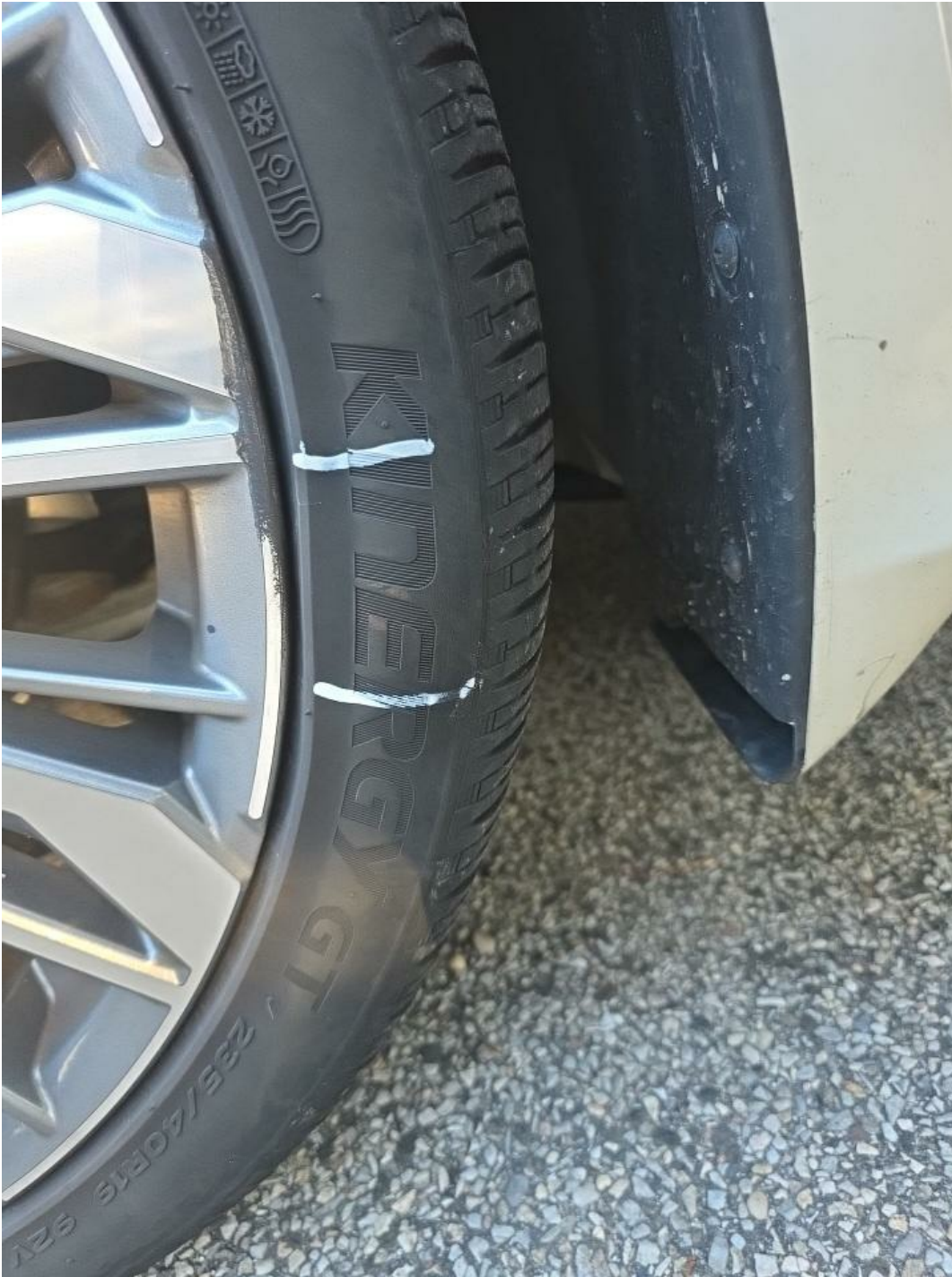
LF Tire Side Wall Bulge Replacement Required
