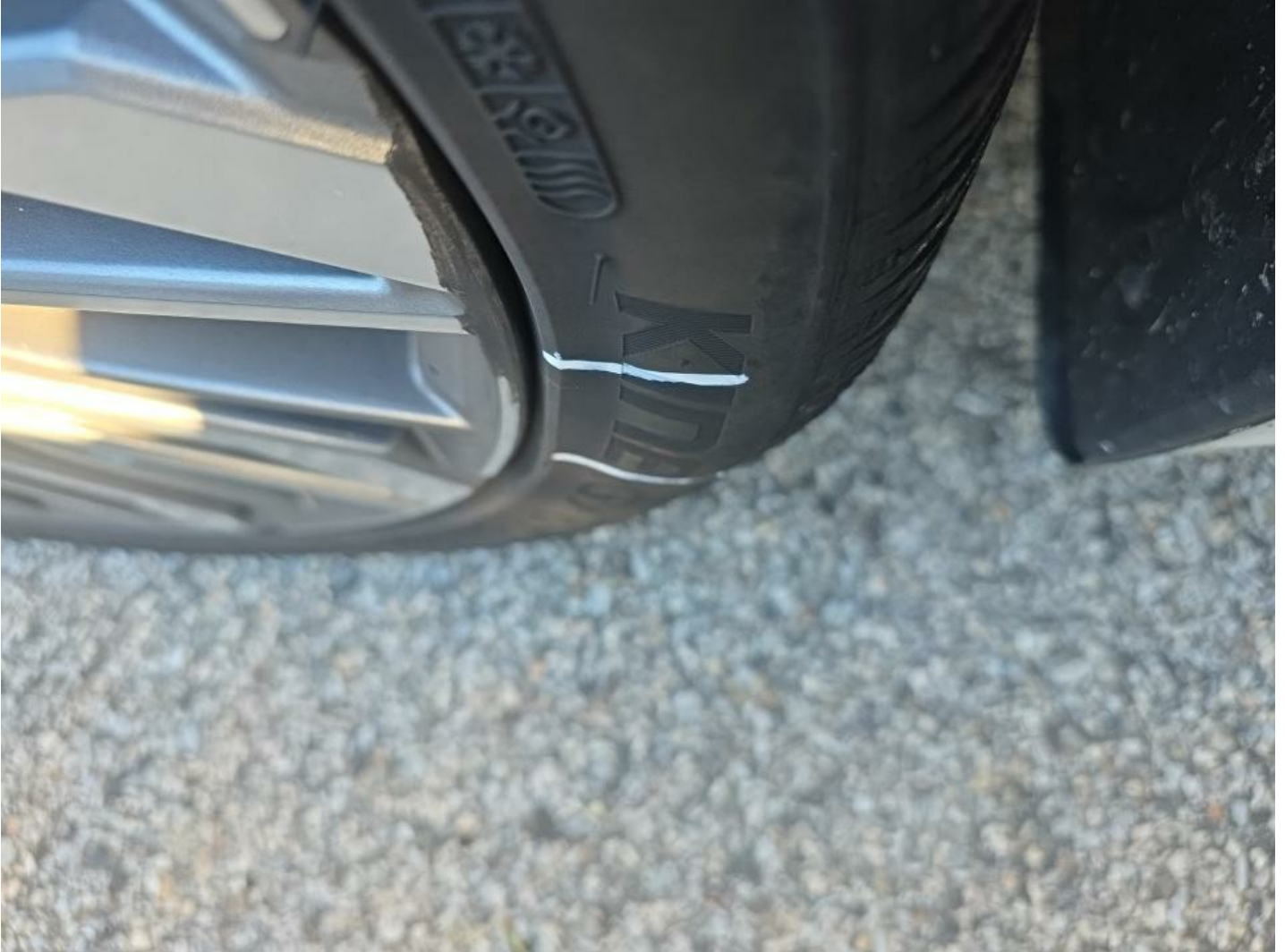
LF Tire Side Wall Bulge Replacement Required
