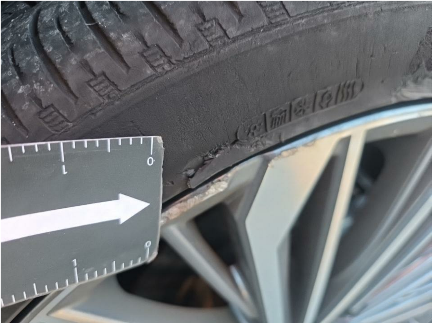
RF Tire Gouged Replacement Required
