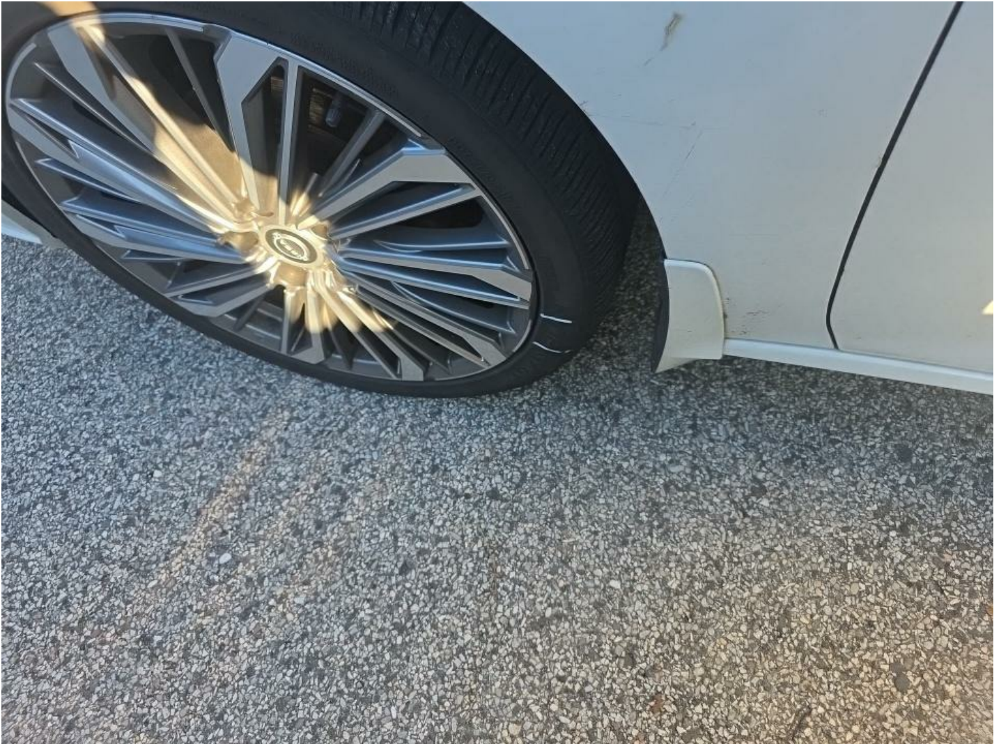
LF Tire Side Wall Bulge Replacement Required
