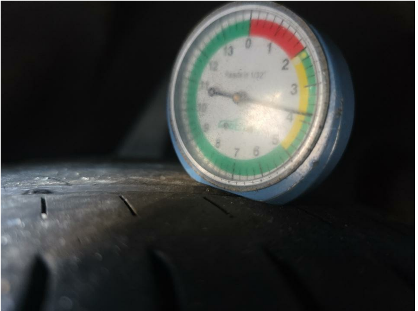
LR Tire Worn Replacement Required
