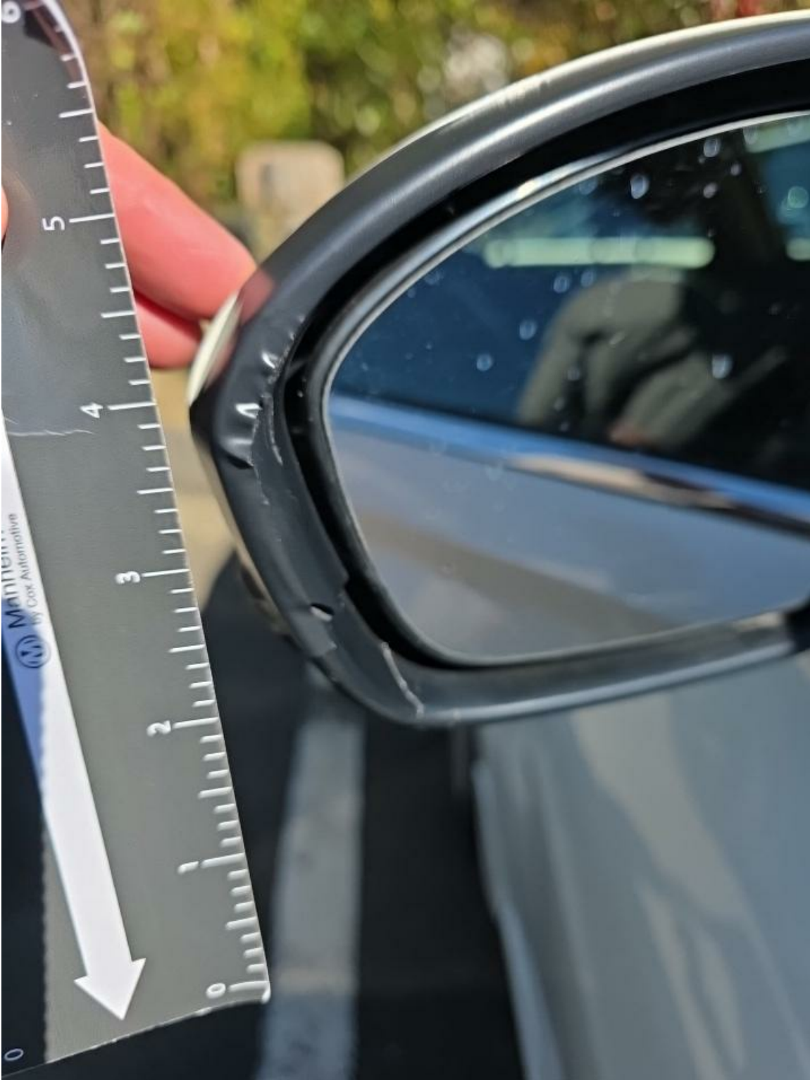
LF Mirror Housing Cracked 2" to 3"
