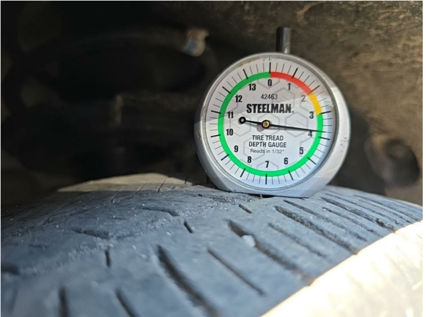
LF Tire Worn Replacement Required
