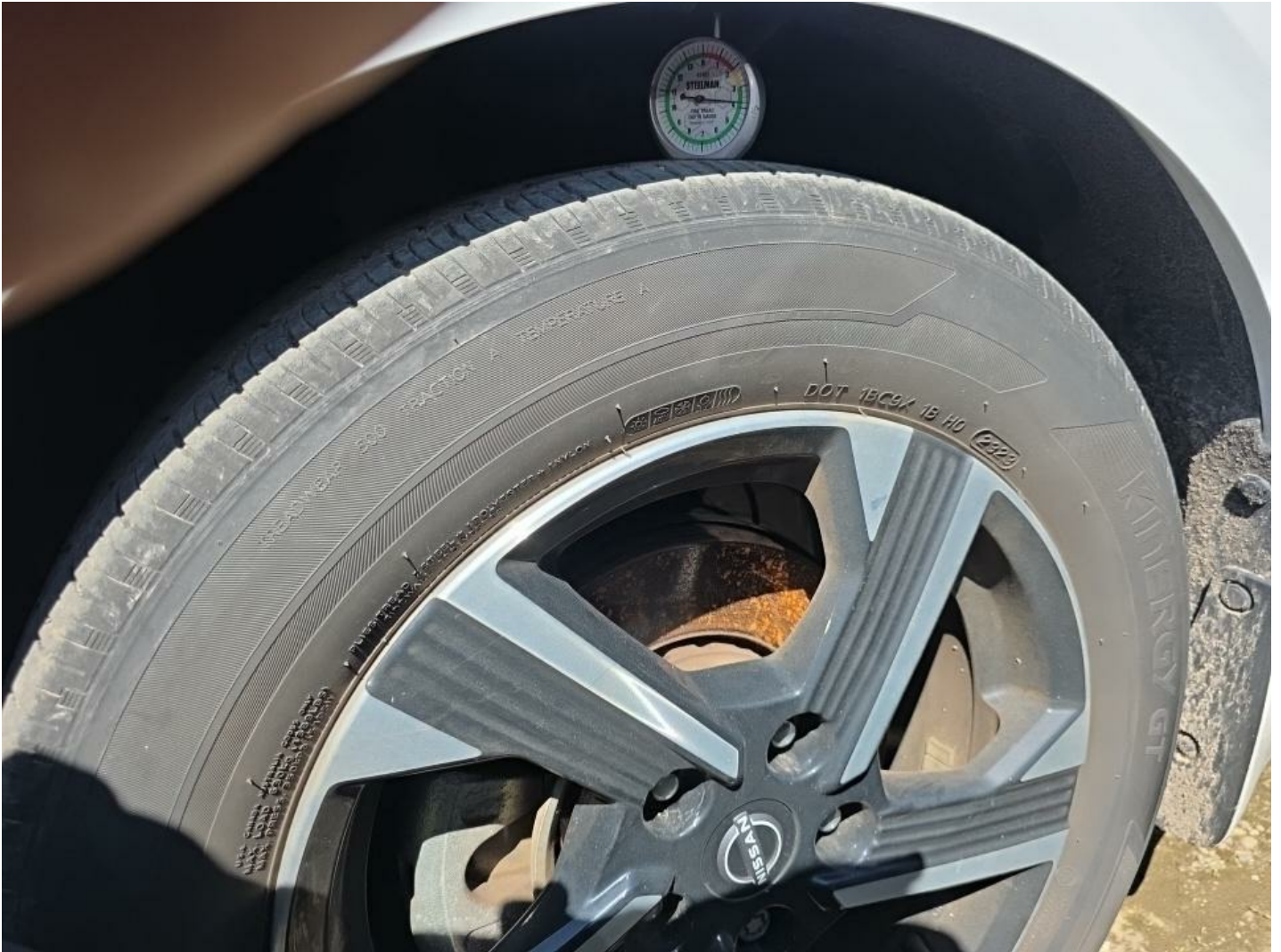
LF Tire Worn Replacement Required
