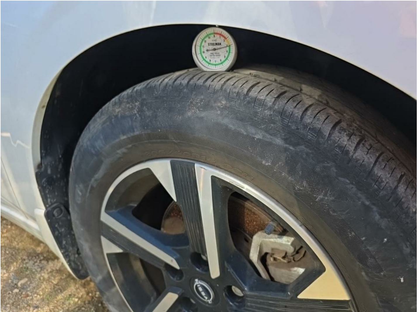
RF Tire Worn Replacement Required
