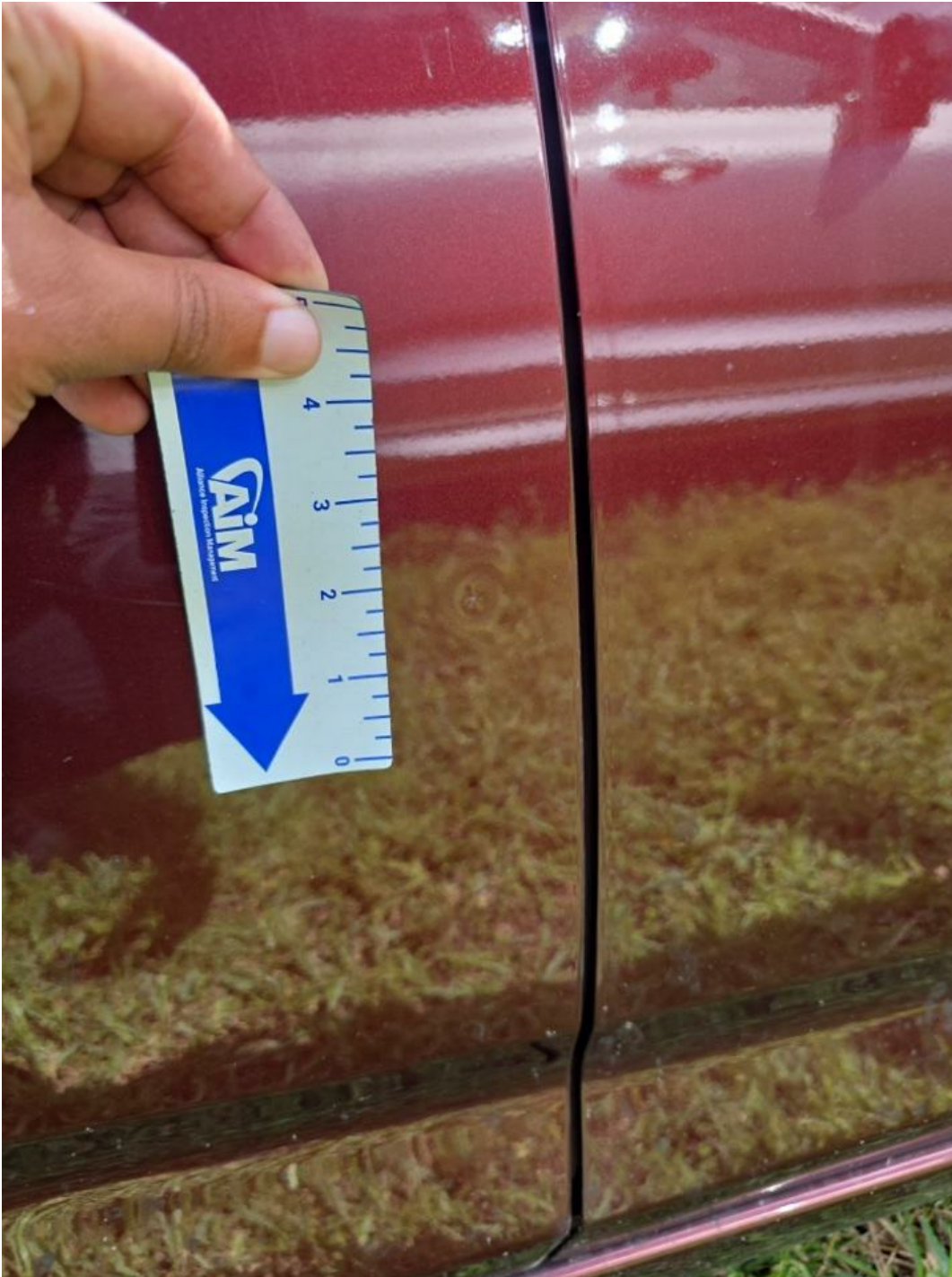
RR Door Dent/No Paint Dmg 1/2" to 1"
