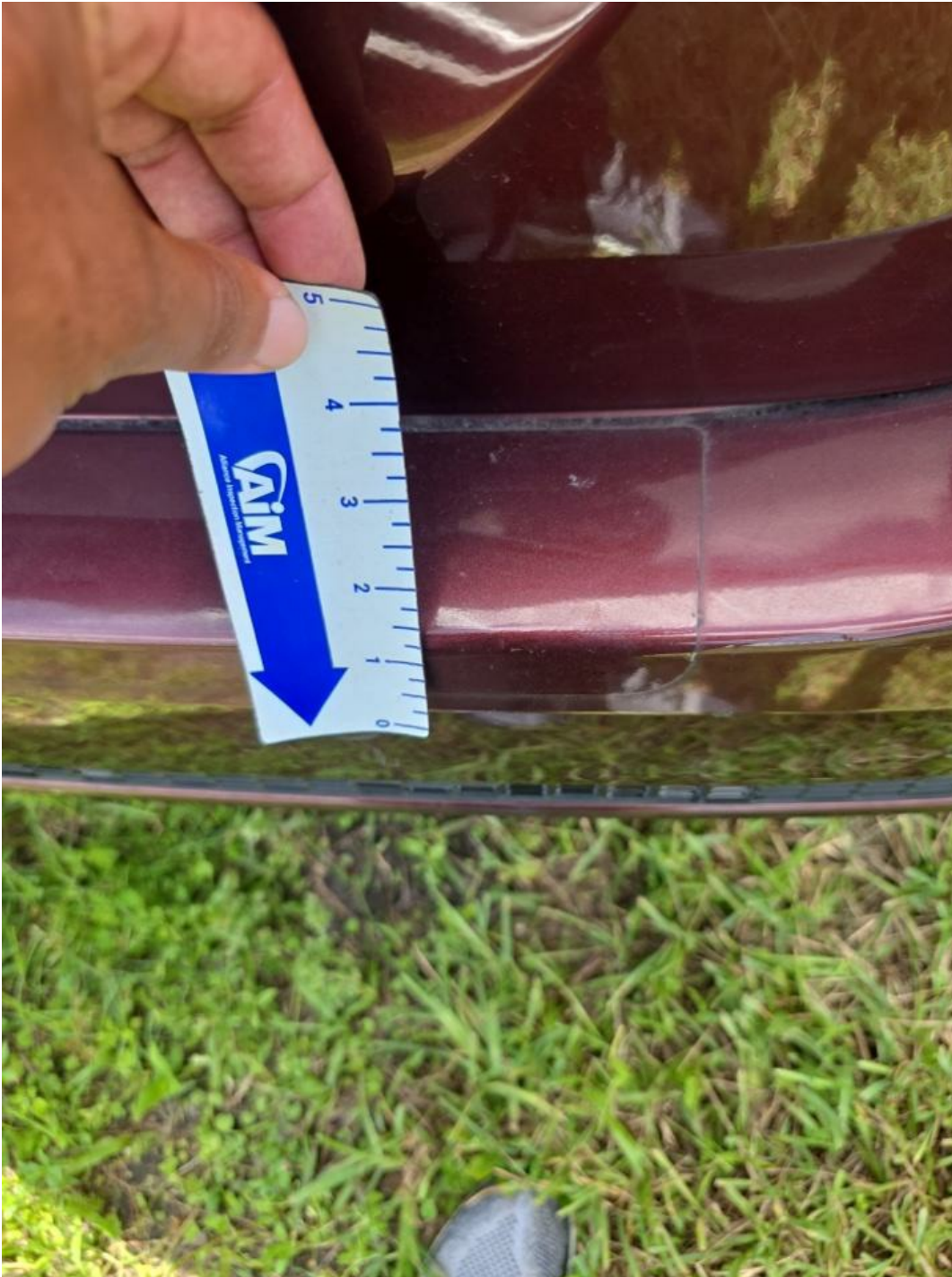
Rear Bumper Dent/No Paint Dmg 1/2" to 1"
