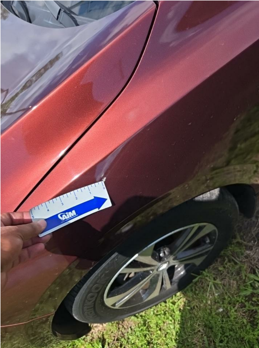
LF Fender Prev Repair Buffable
