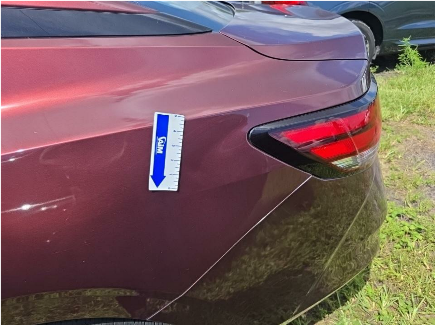
L Qtr Panel Dent/No Paint Dmg 8" to 9"
