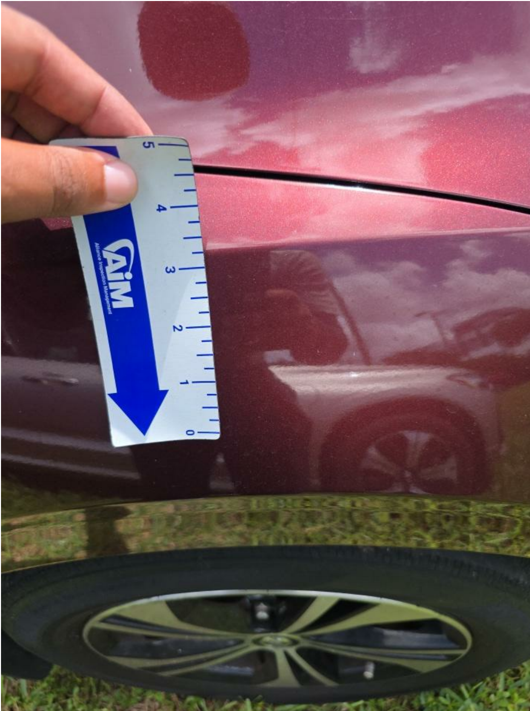
RF Fender Dent/No Paint Dmg 1/2" to 1"
