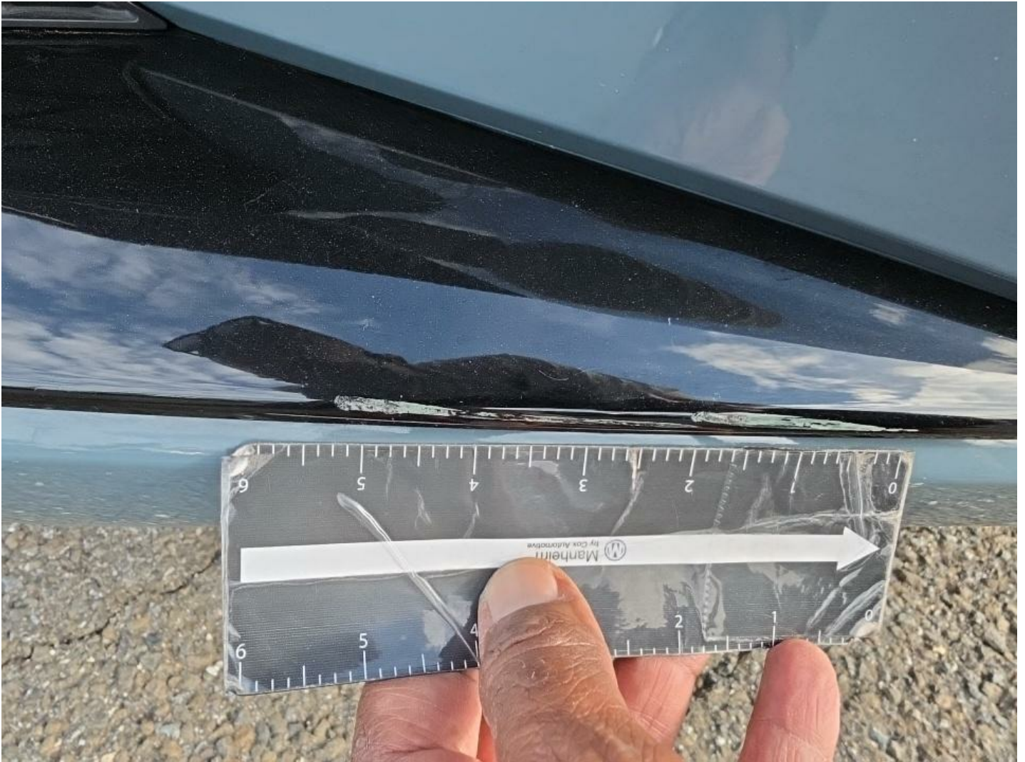
Right Fog Light Covers Scratch Heavy 5" to 6"
