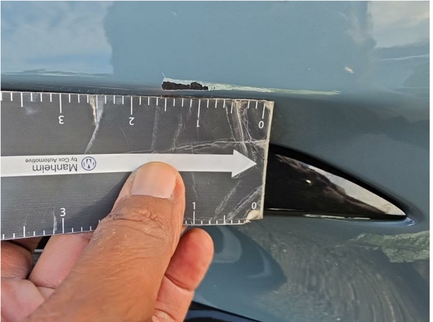
Front Bumper Scratch Heavy 1" to 2"
