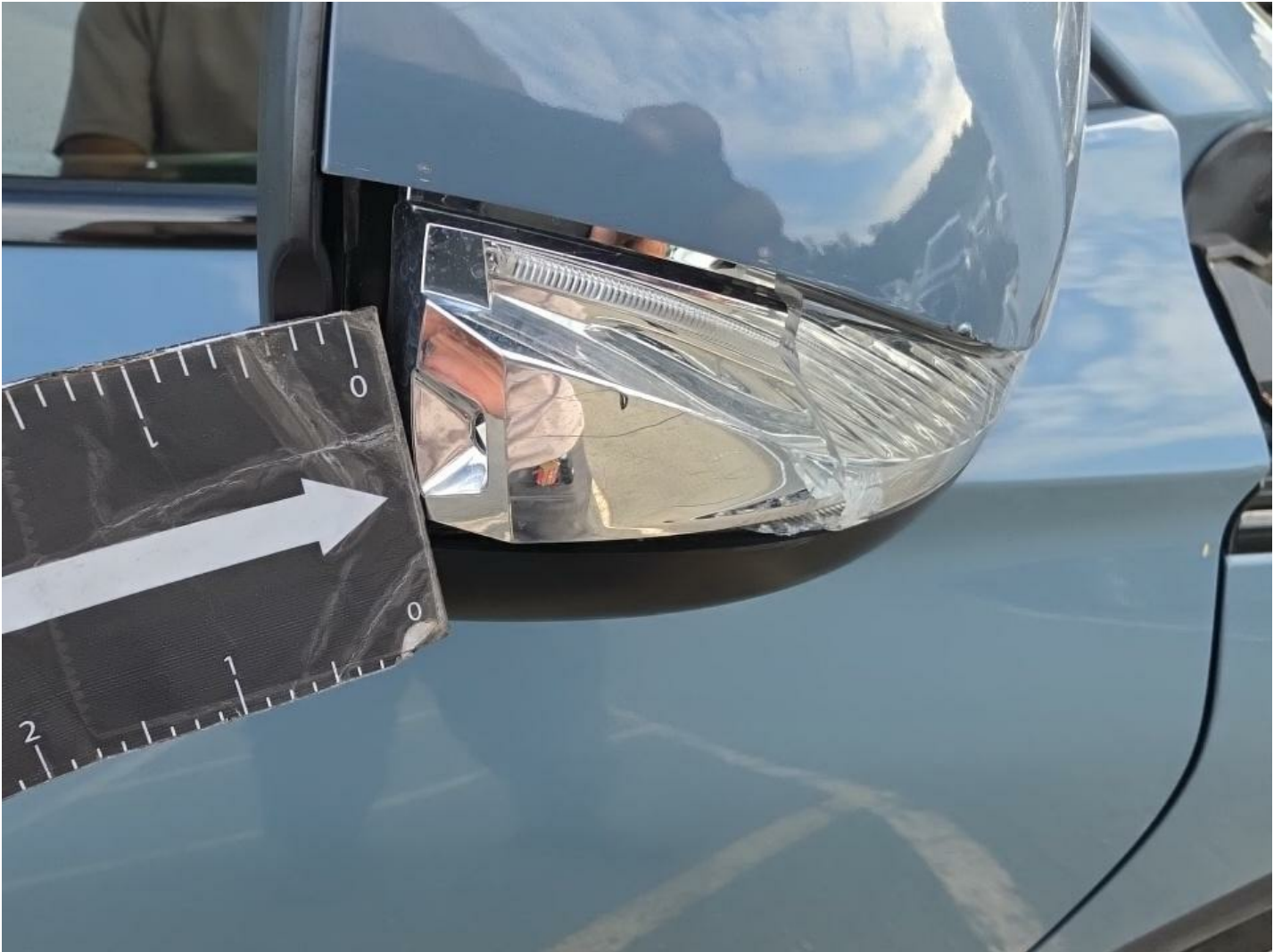
RF Turn Signal Broken Replacement Required
