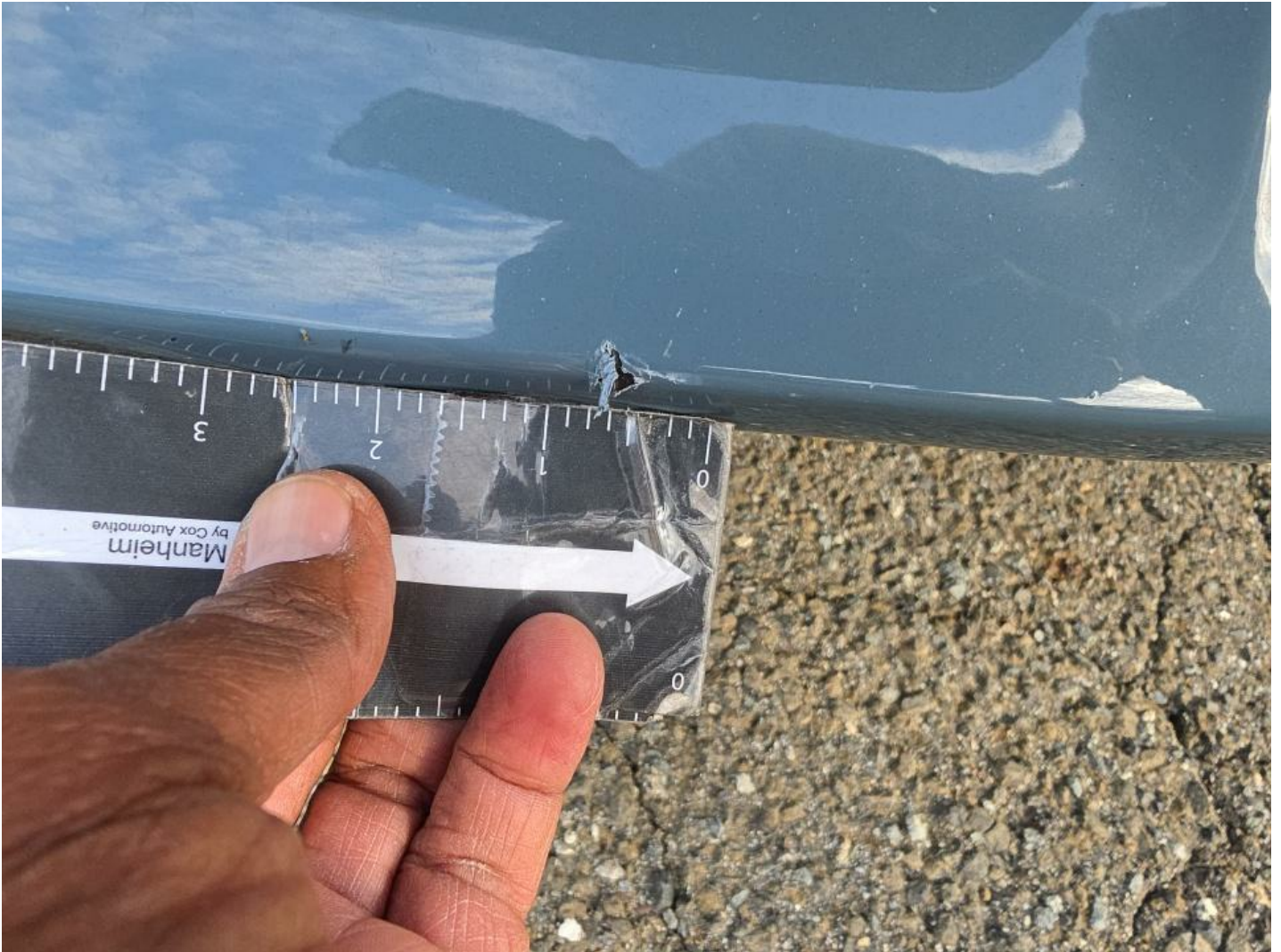
Front Bumper Gouged 1/2" to 1"
