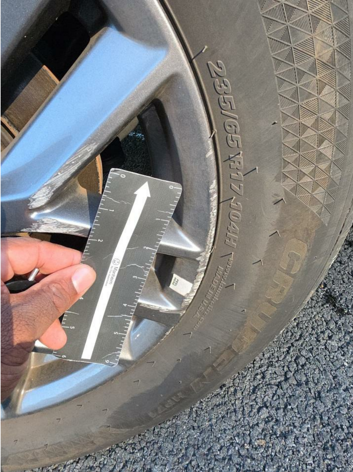
LF Wheel Curb Rash 5" to 6"
