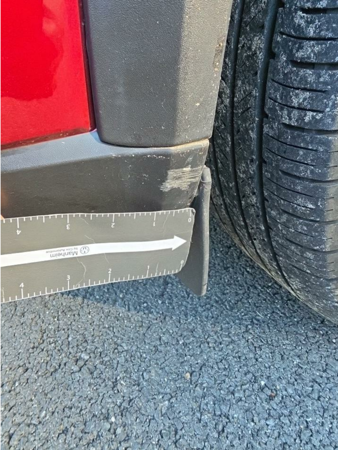
F Bumper Molding Scratch Heavy 1" to 2"
