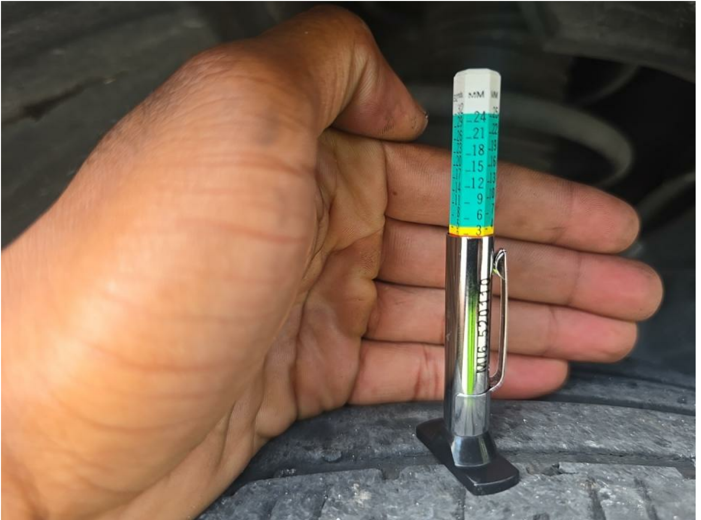
LF Tire Worn Replacement Required
