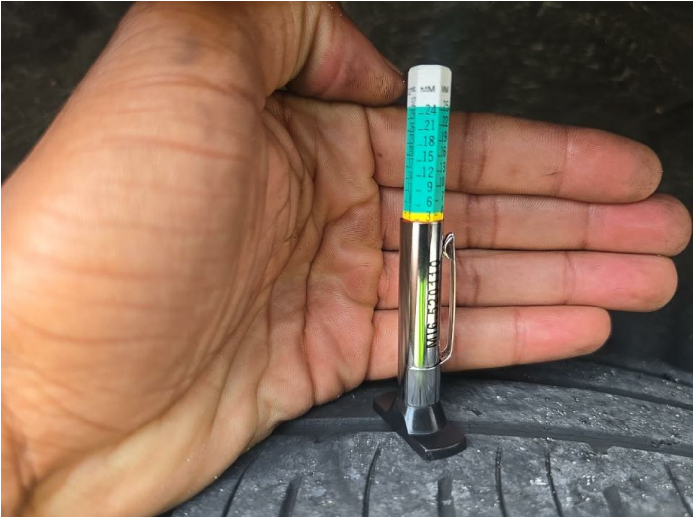
LR Tire Worn Replacement Required
