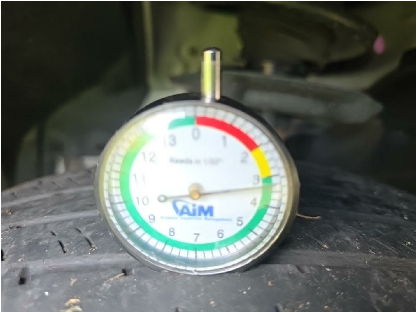
LF Tire Worn Replacement Required
