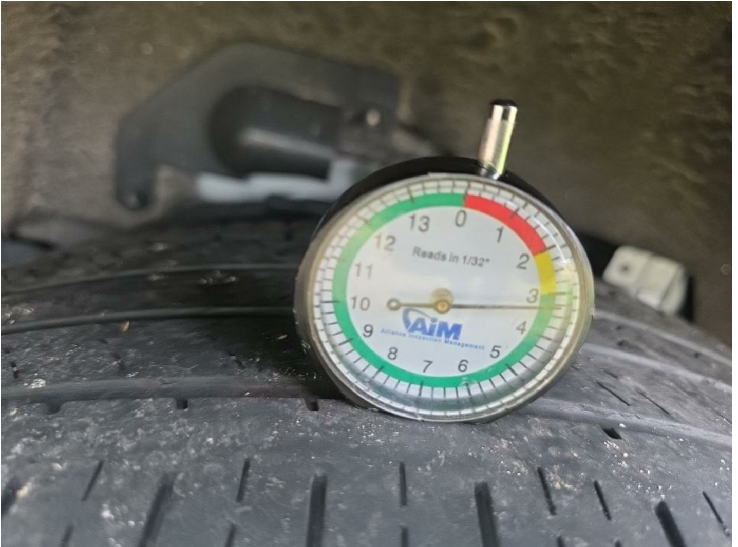
RR Tire Worn Replacement Required
