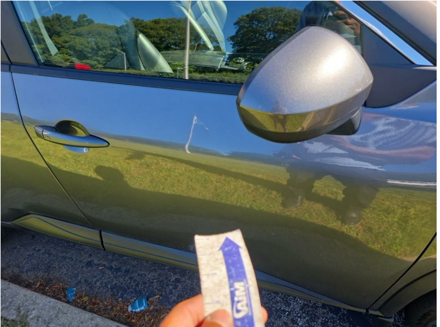
RF Door Prev Repair Acceptable
