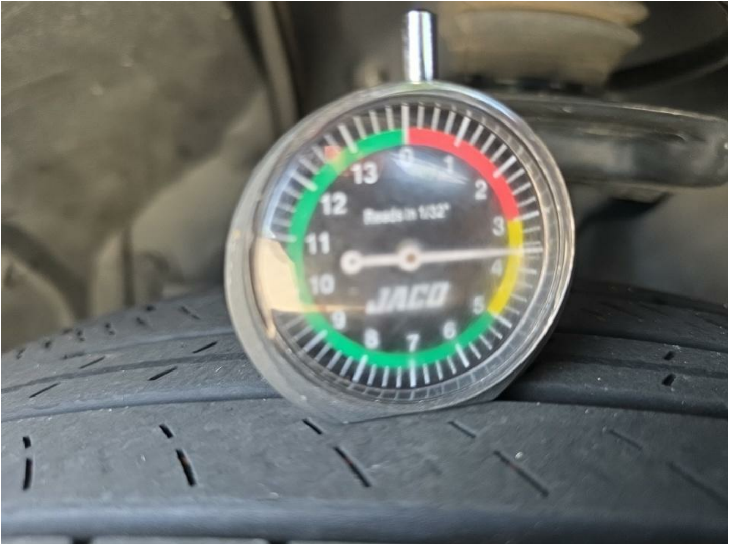
LF Tire Worn Replacement Required
