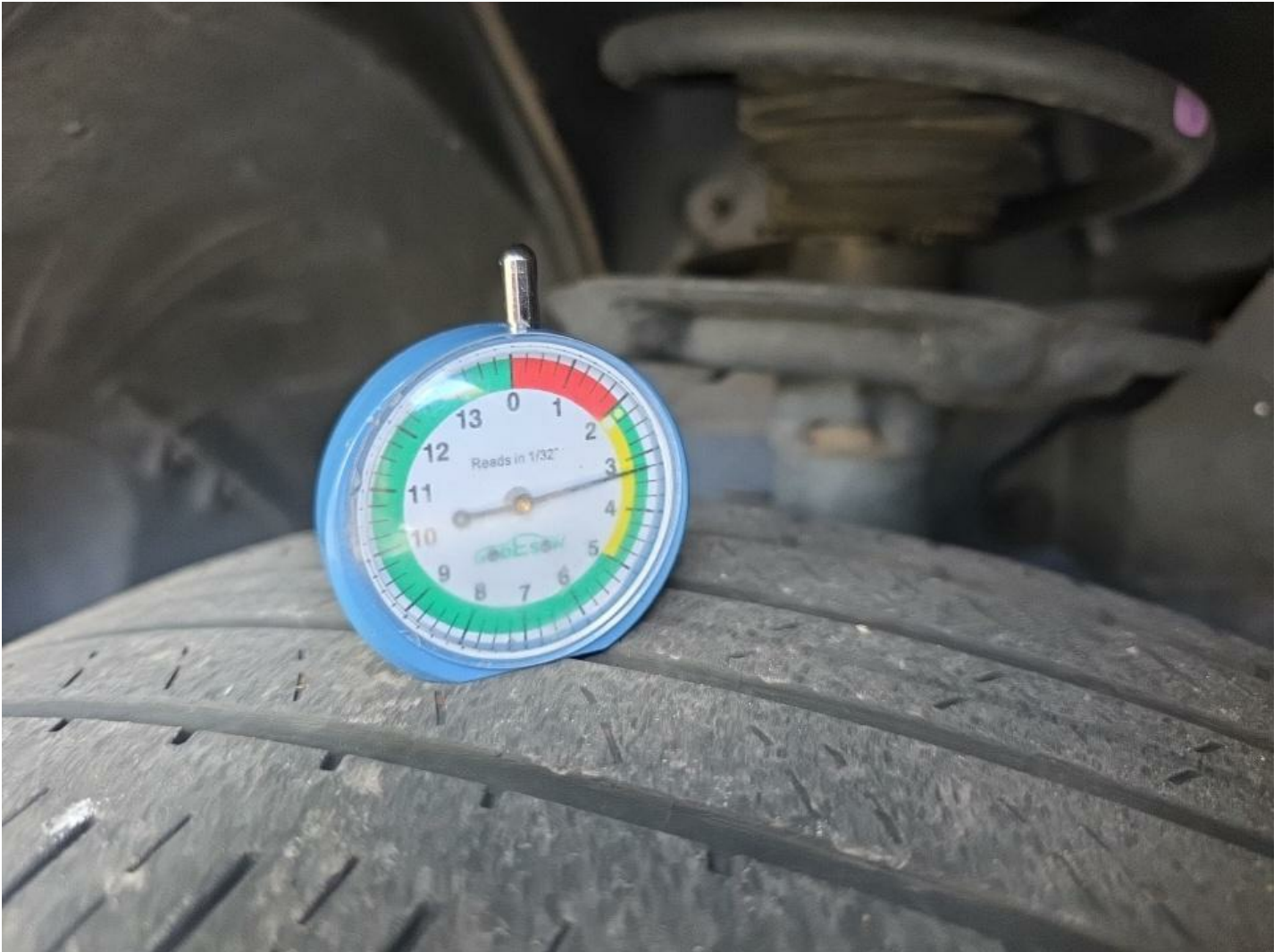
LF Tire Worn Replacement Required
