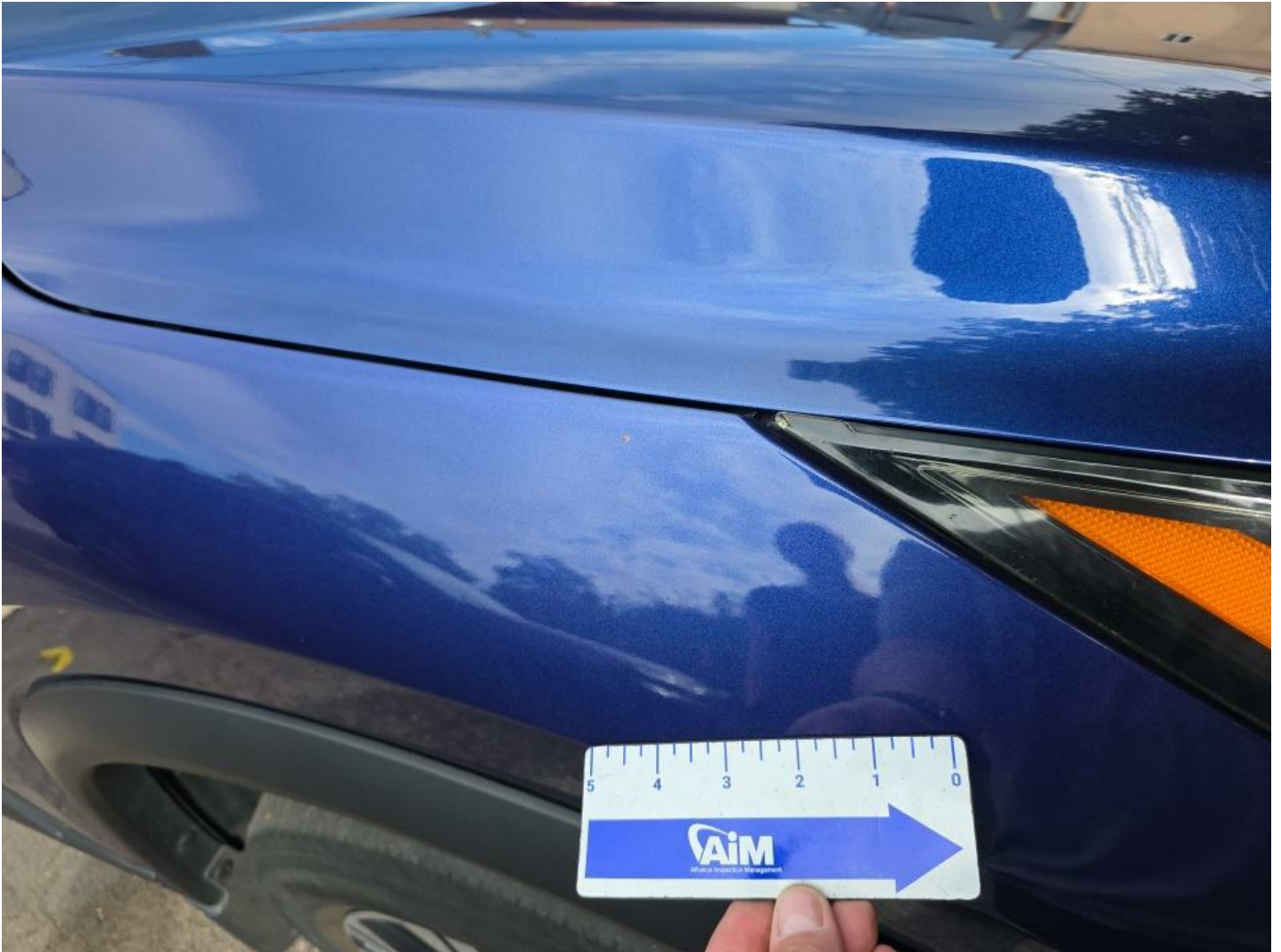
RF Fender Prev Repair Acceptable
