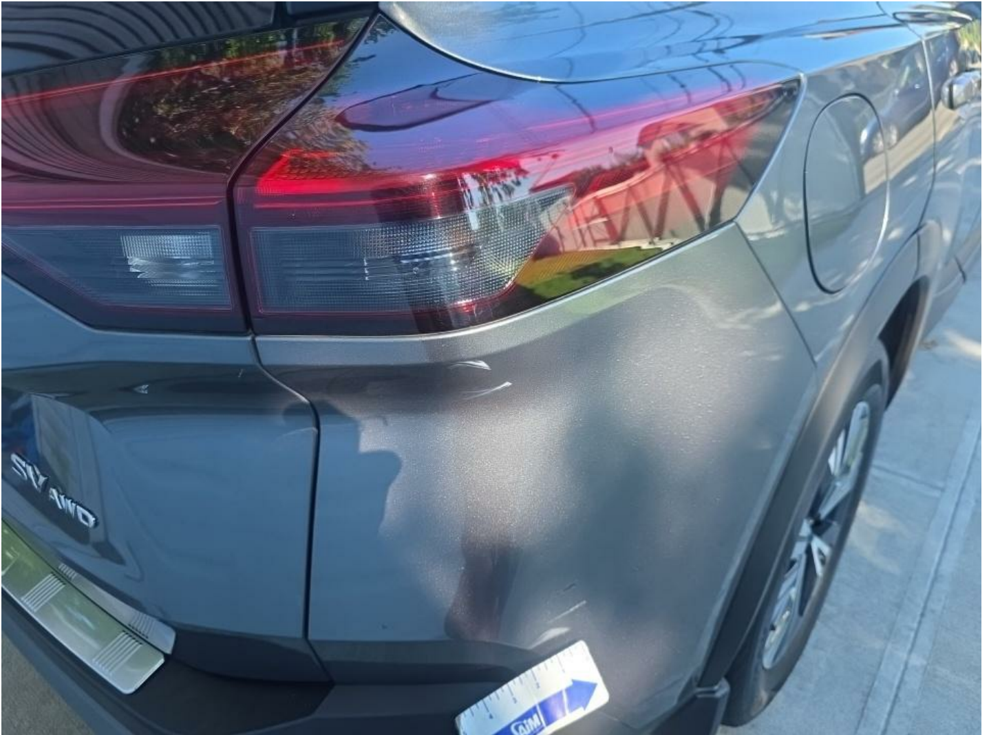
Rear Bumper Scratch Heavy 2" to 3"
