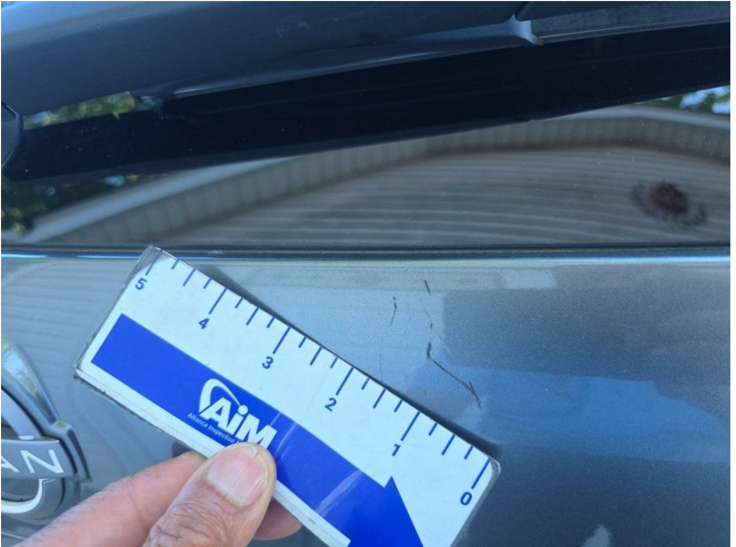
Lift Gate Scratch Heavy 2" to 3"
