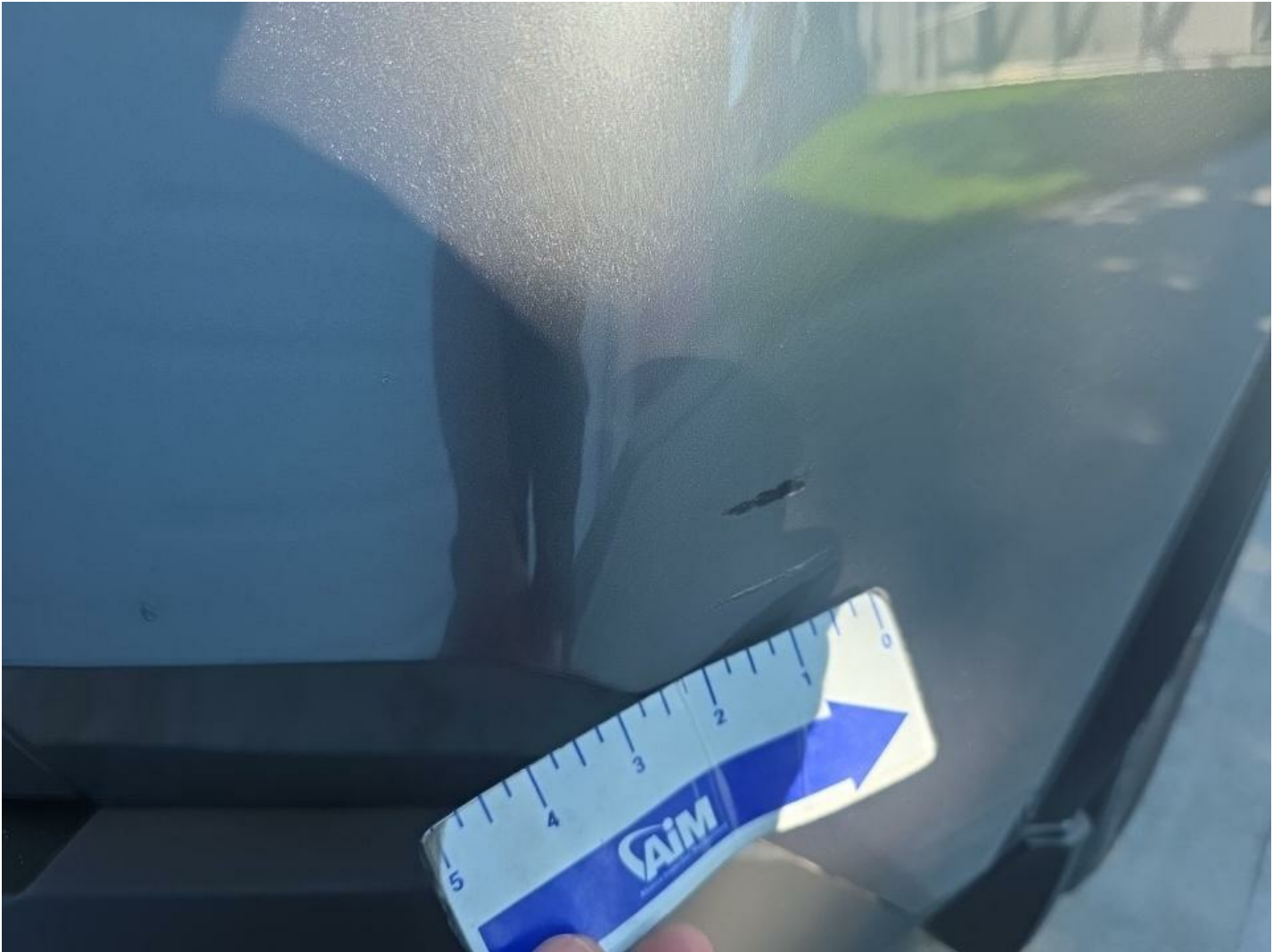
Rear Bumper Scratch Heavy 2" to 3"
