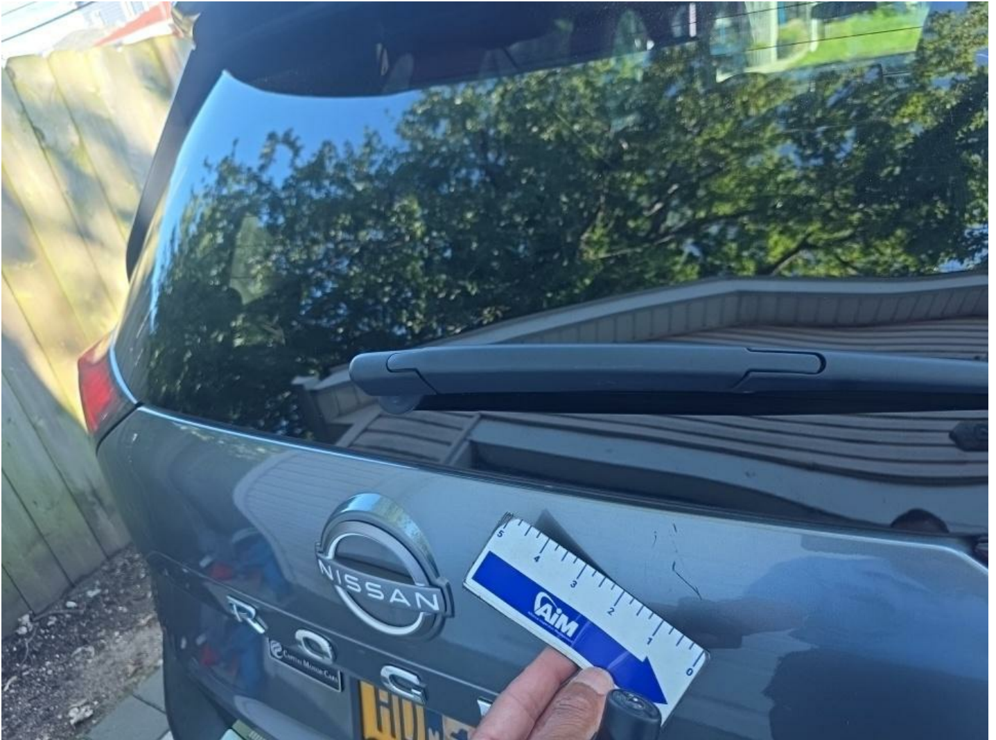
Lift Gate Scratch Heavy 2" to 3"
