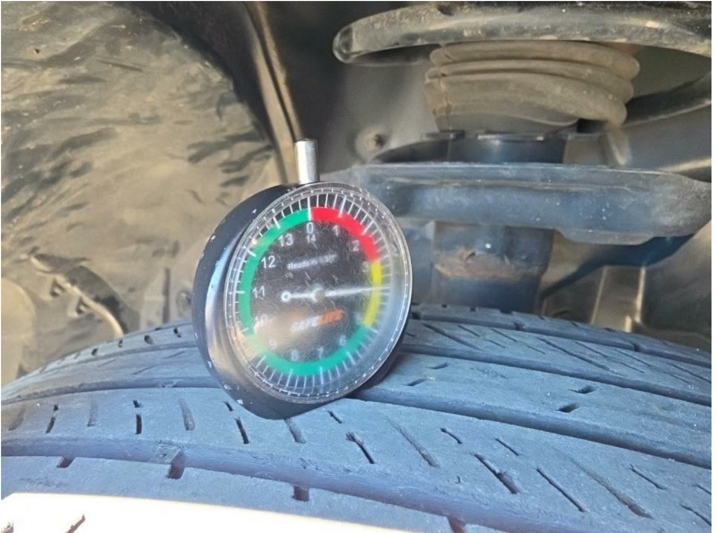
LF Tire Worn Replacement Required
