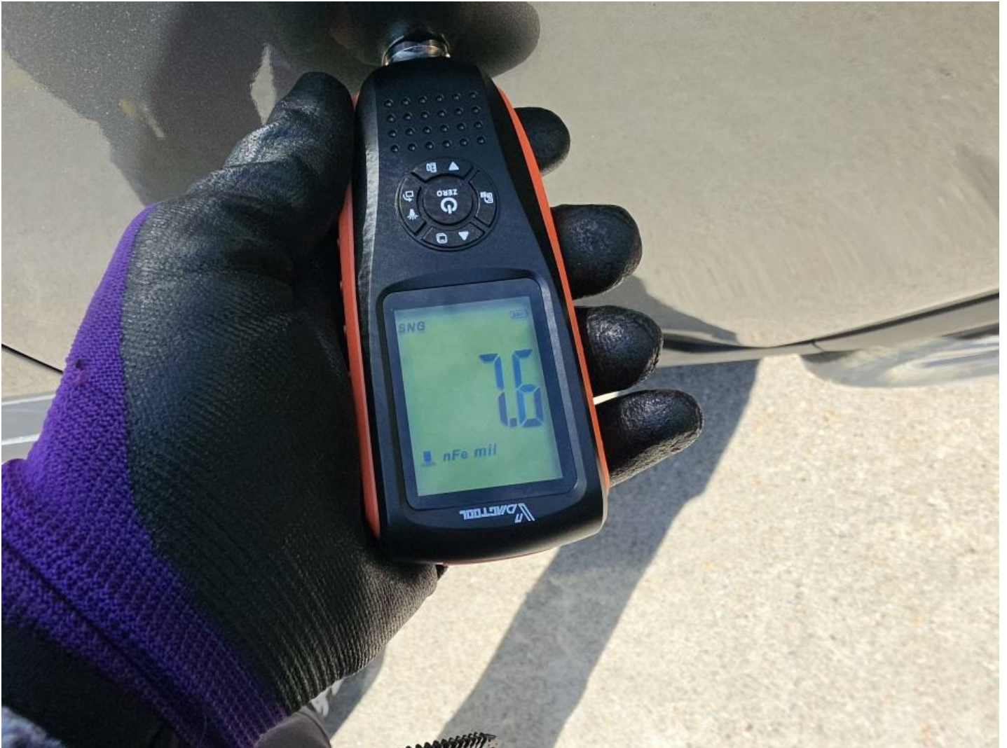
LR Door Prev Repair Acceptable
