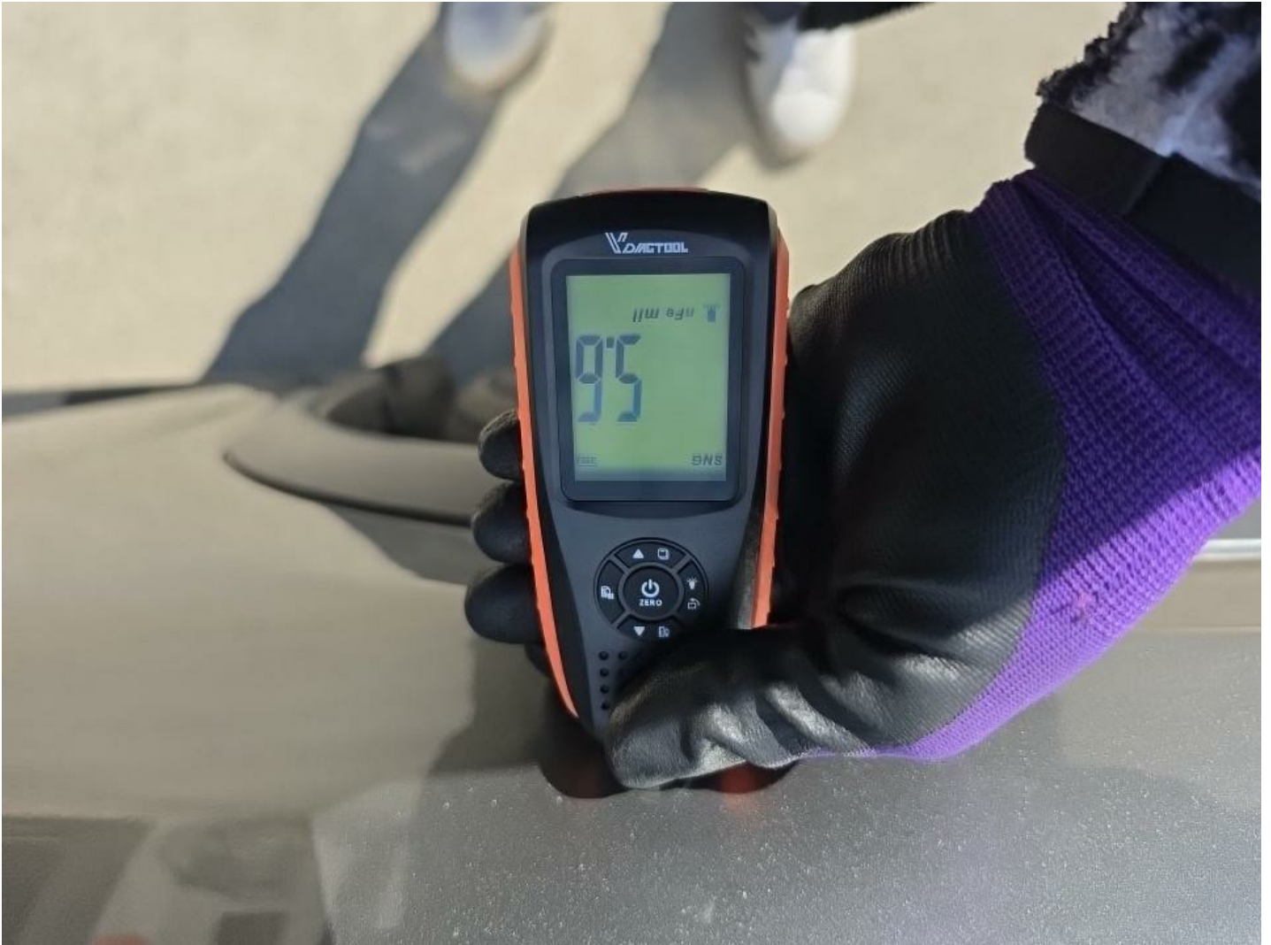
LF Fender Prev Repair Acceptable
