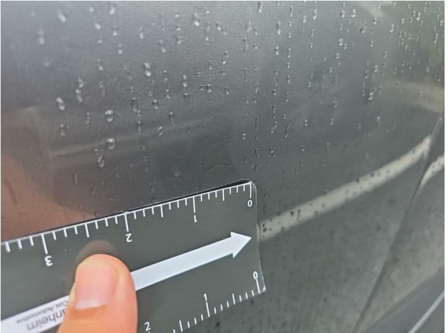
LF Door Dent/Paint Dmg 1/8" to 1/2"
