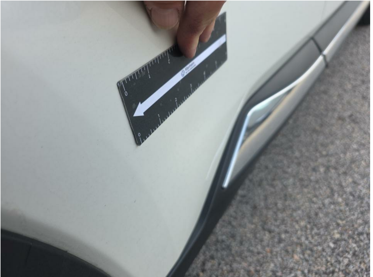
RR Door Dent/No Paint Dmg 5" to 6"
