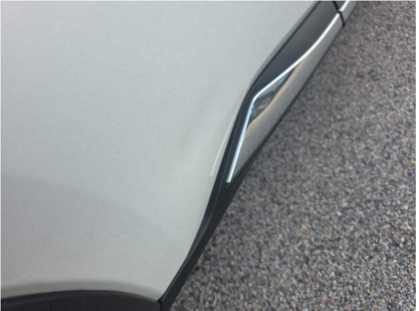
RR Door Dent/No Paint Dmg 5" to 6"
