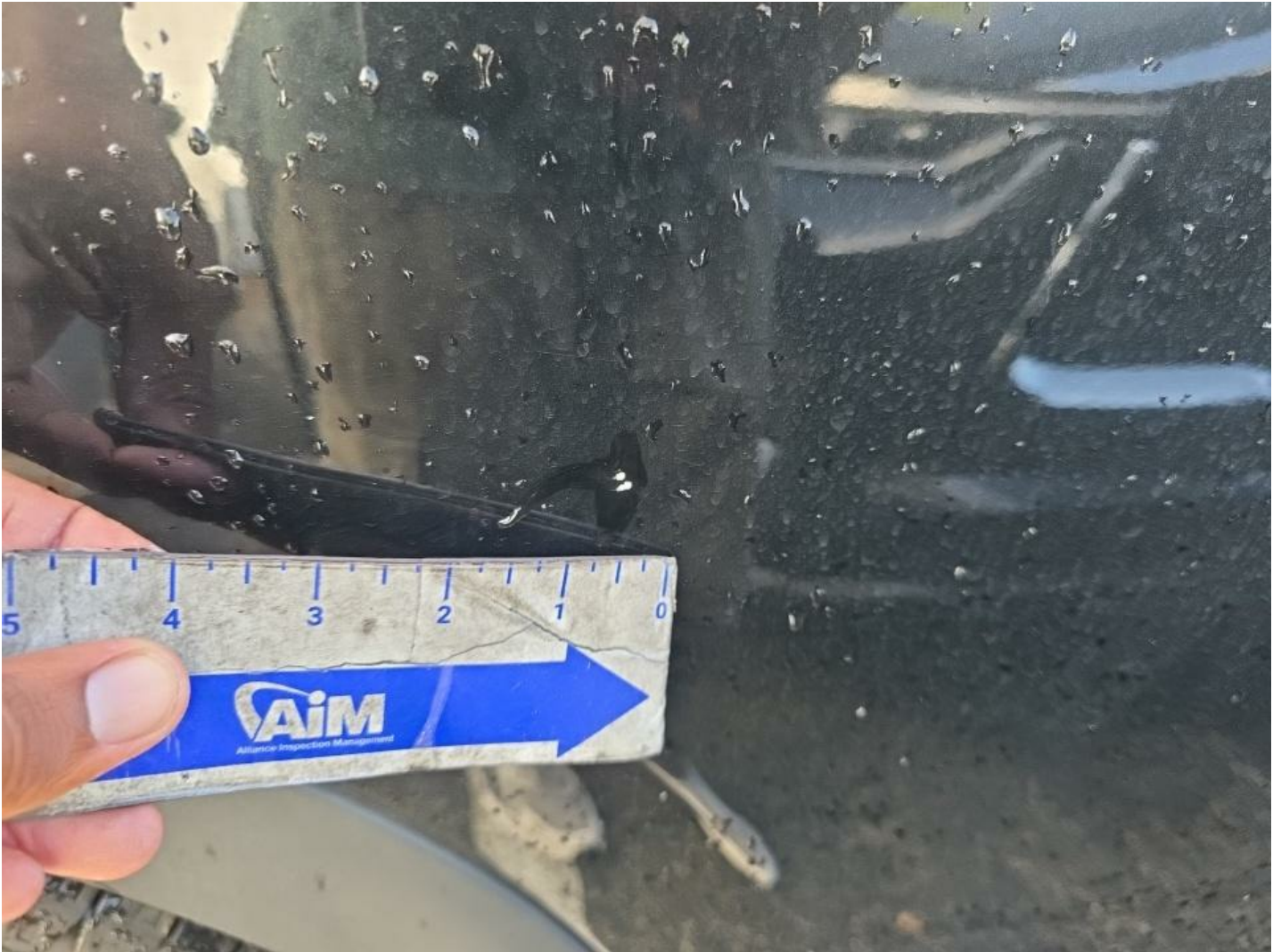
RR Door Dent/Paint Dmg < 1/8"
