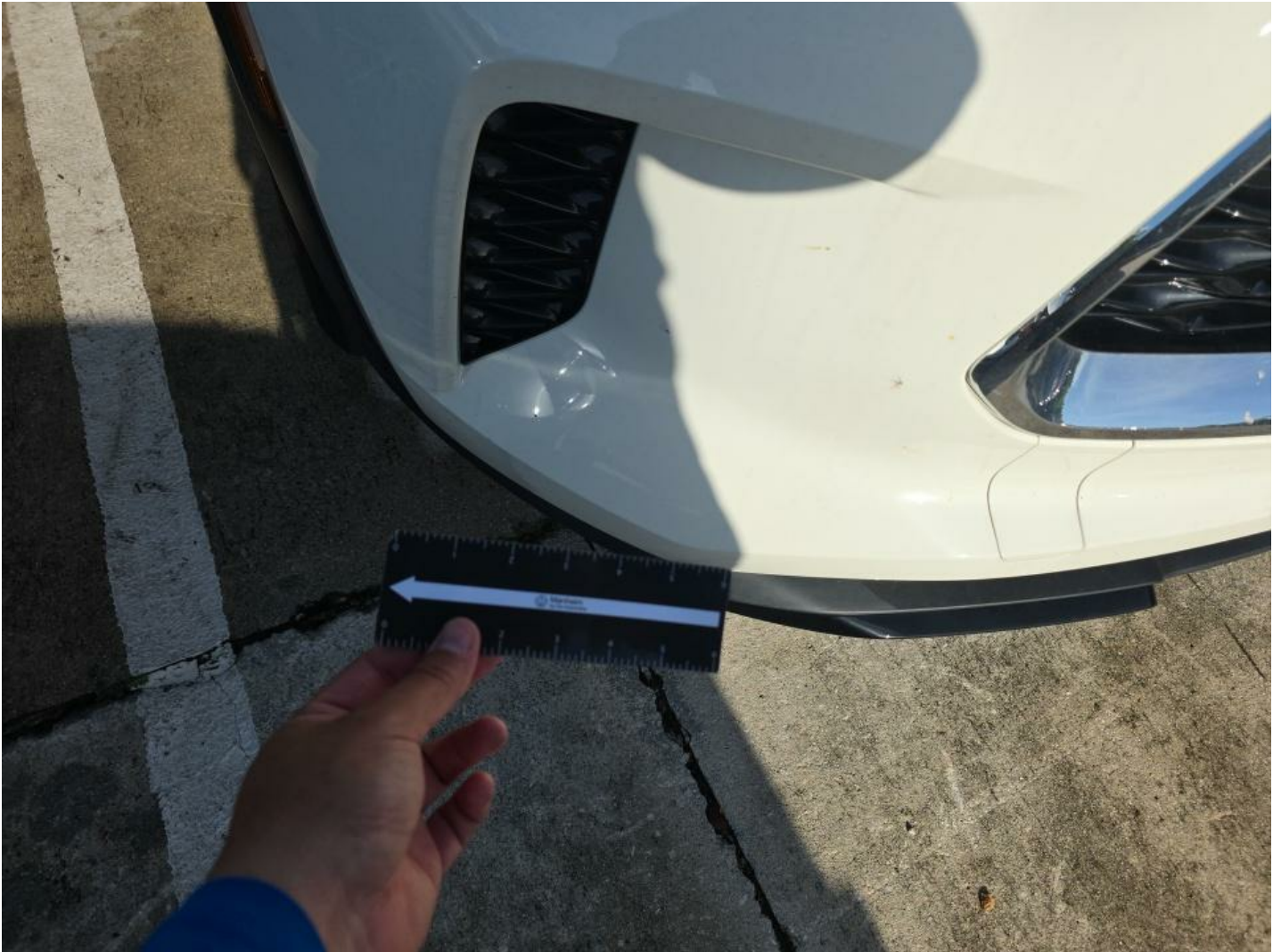
Front Bumper Chipped 2
