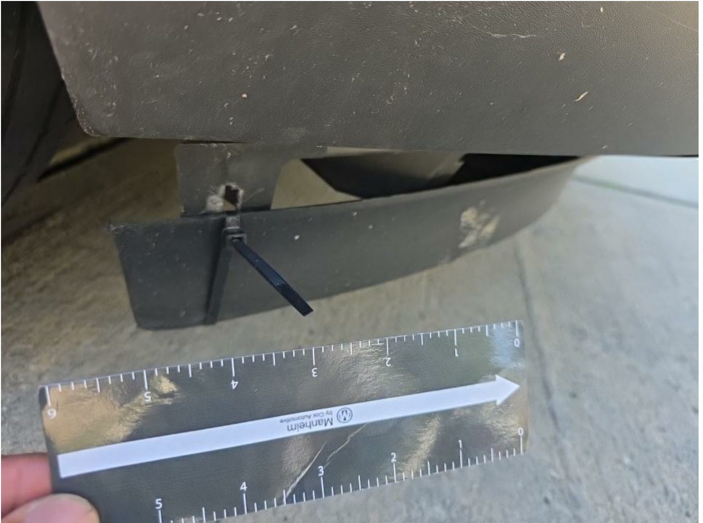
Front Air Dam Loose Repair Required
