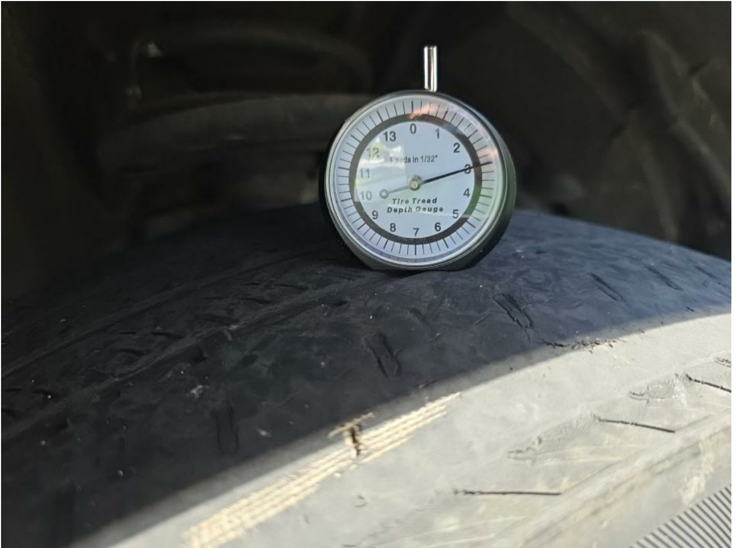
LF Tire Worn Replacement Required
