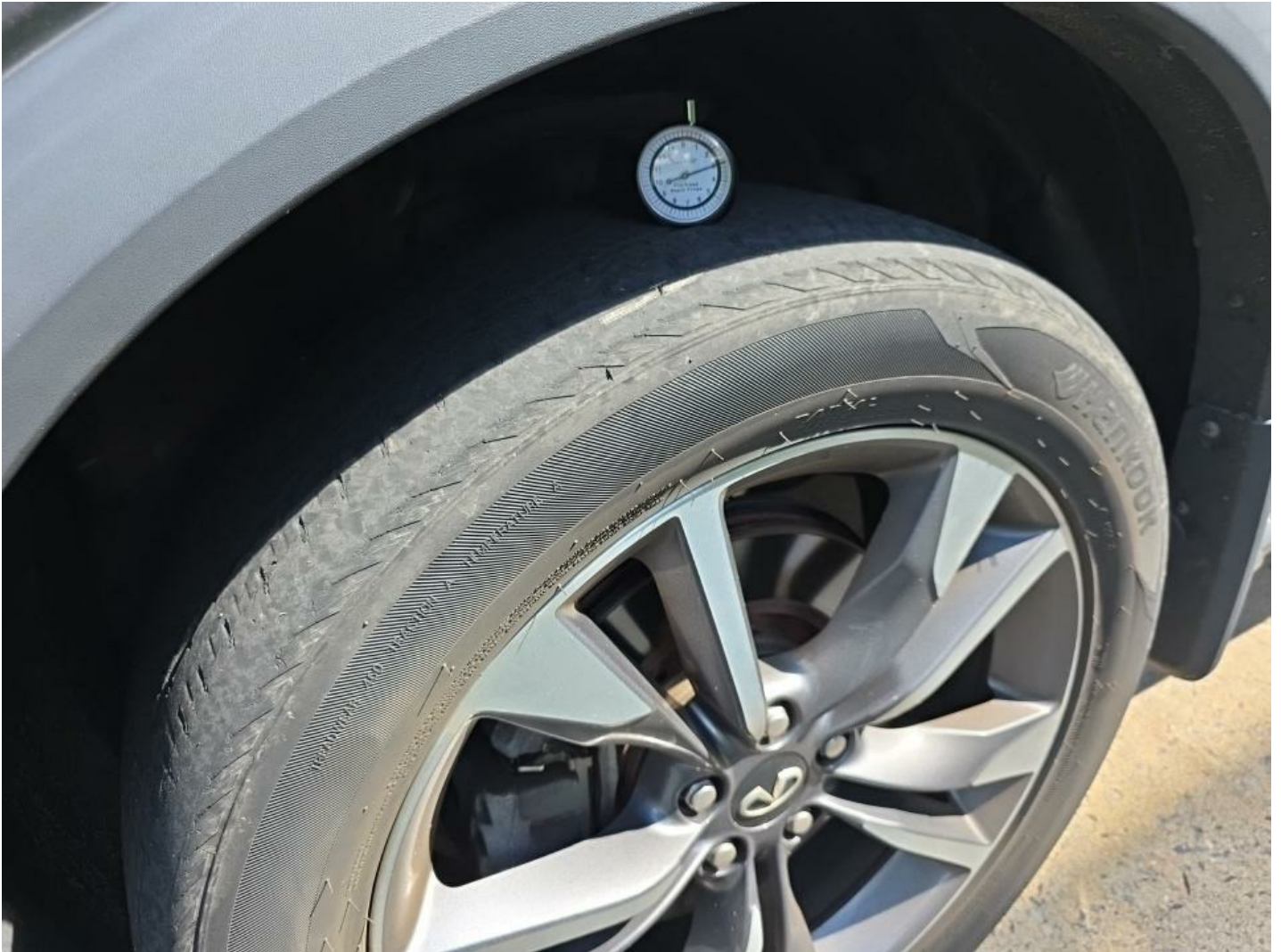
LF Tire Worn Replacement Required
