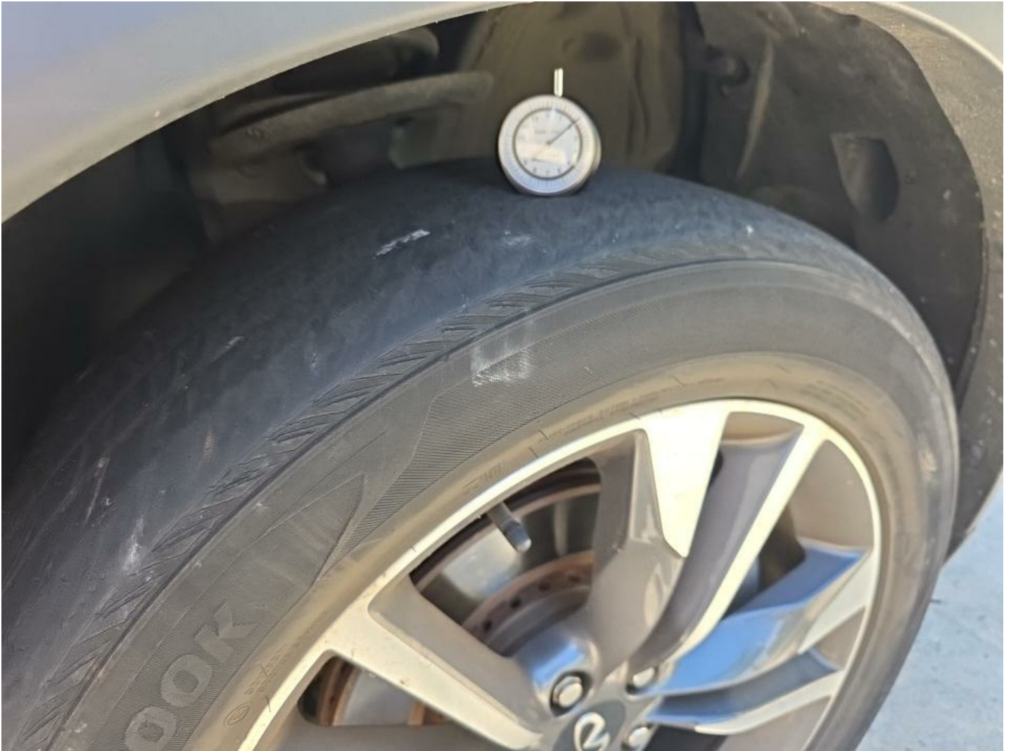
RF Tire Worn Replacement Required
