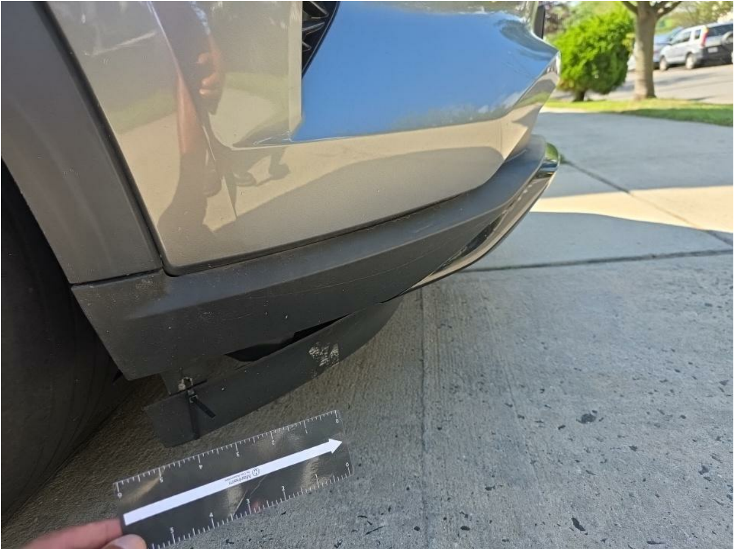
Front Air Dam Loose Repair Required
