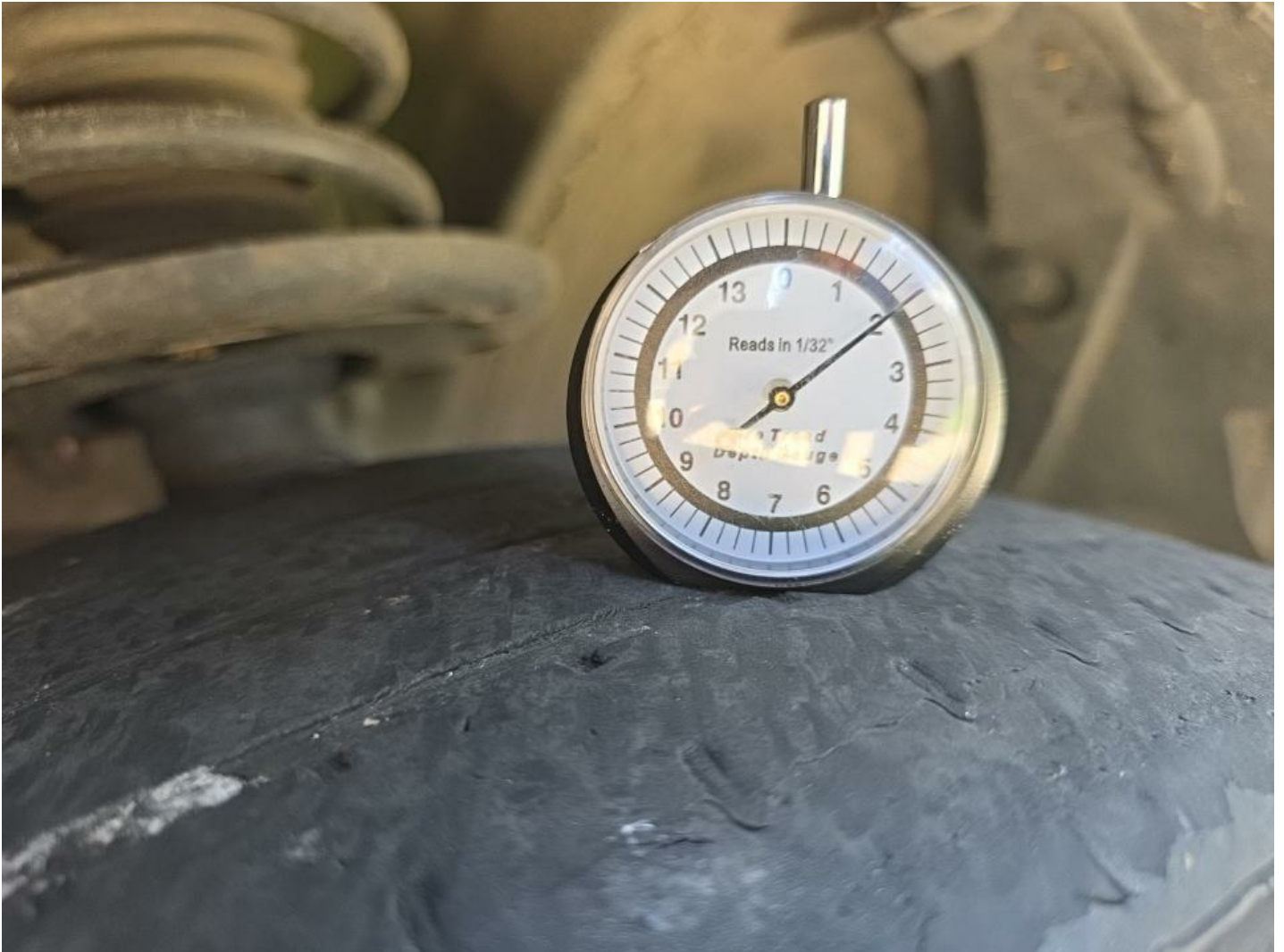
RF Tire Worn Replacement Required
