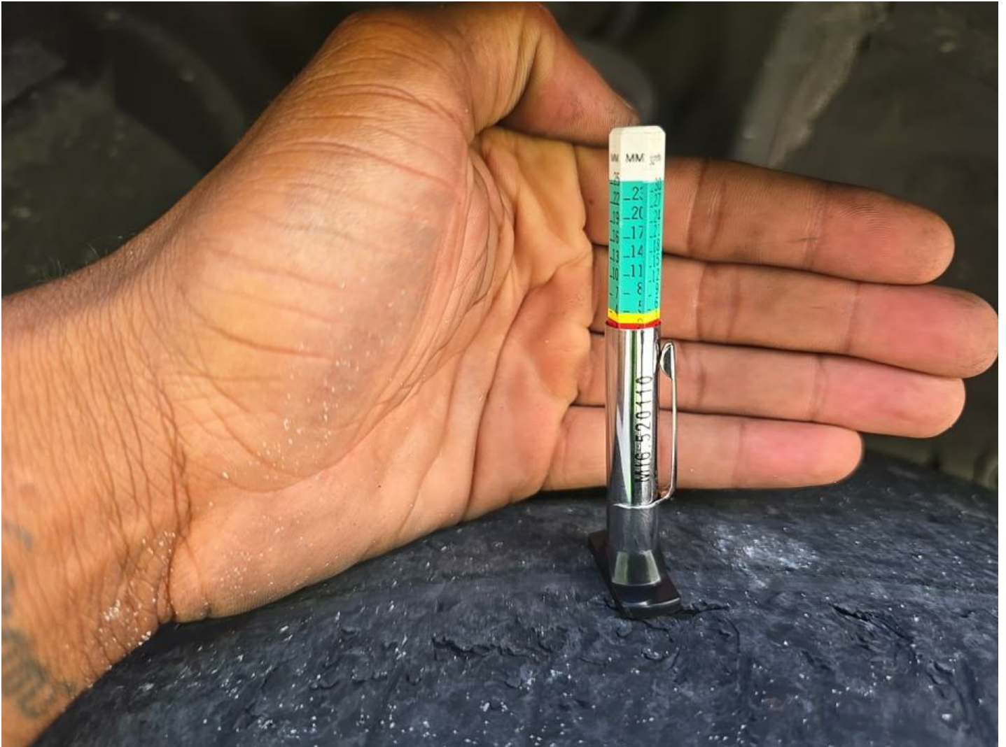
RF Tire Worn Replacement Required
