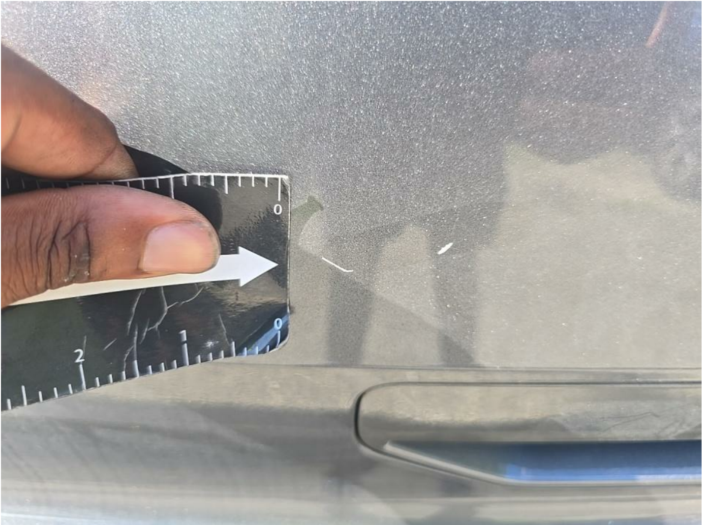
Lift Gate Chipped 2
