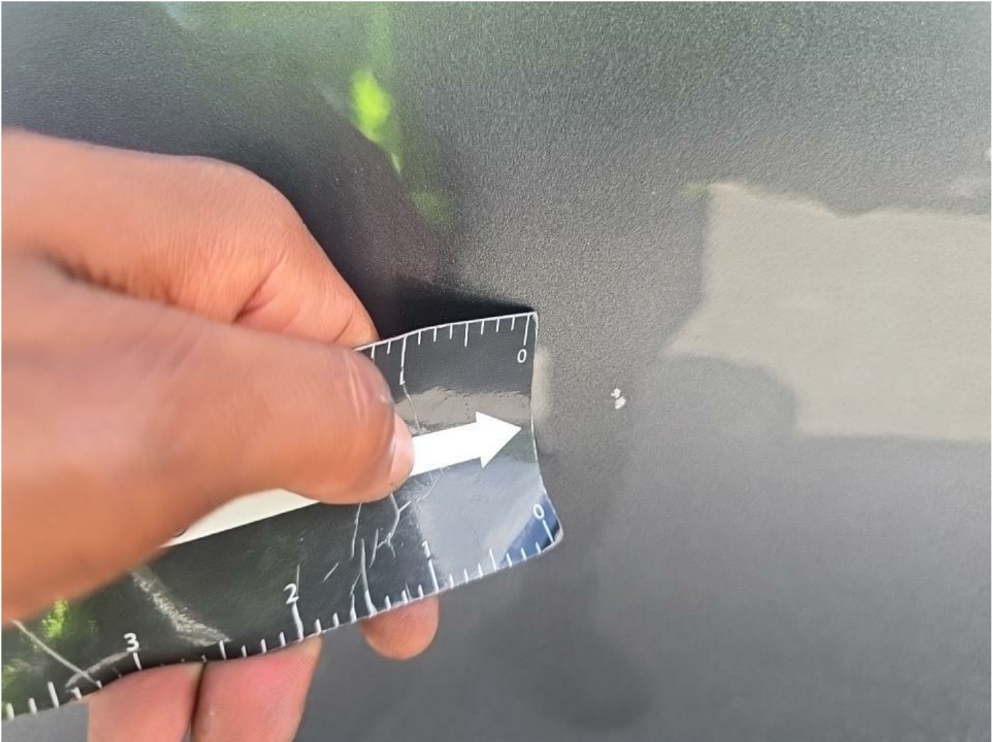
RR Door Chipped 1
