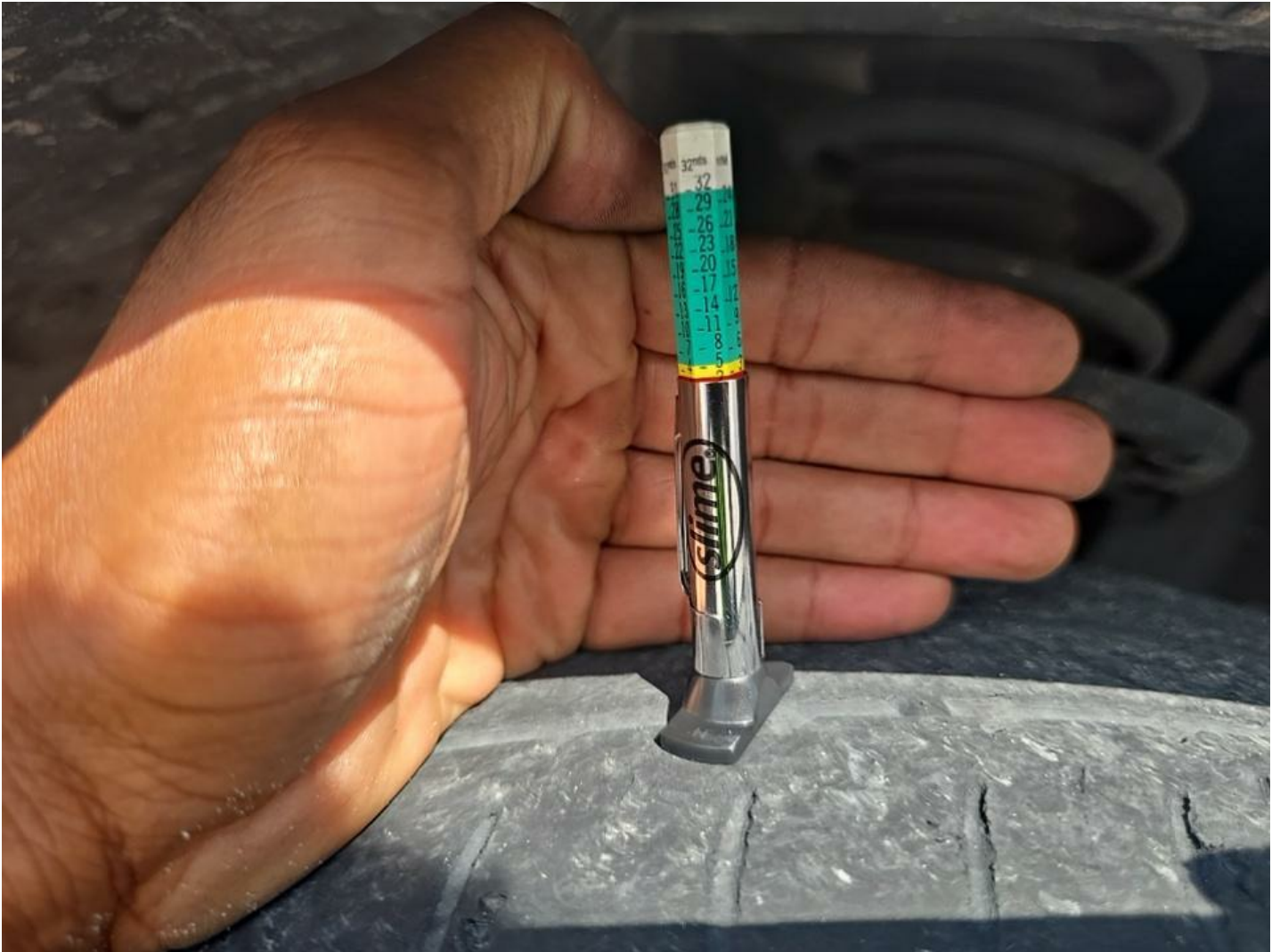
LF Tire Worn Replacement Required
