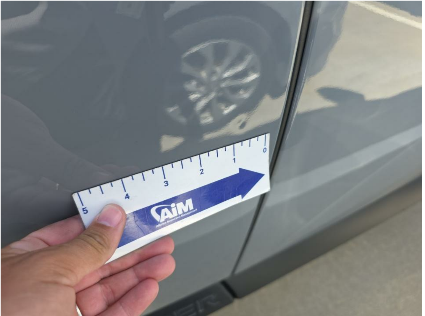
RR Door Dent/No Paint Dmg 1/2" to 1"
