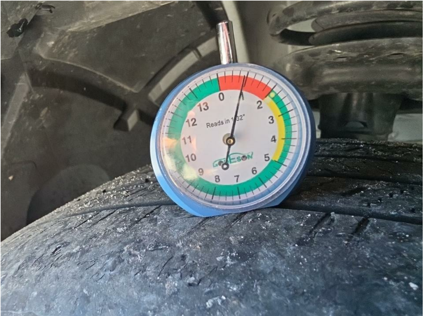
LF Tire Worn Replacement Required
