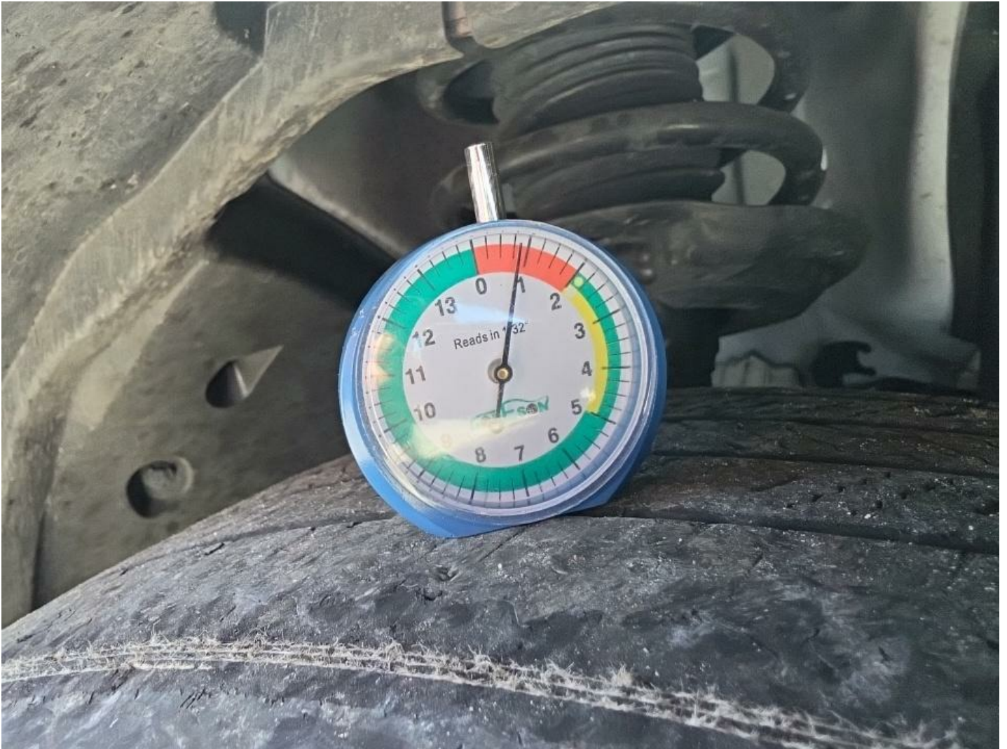
RF Tire Worn Replacement Required
