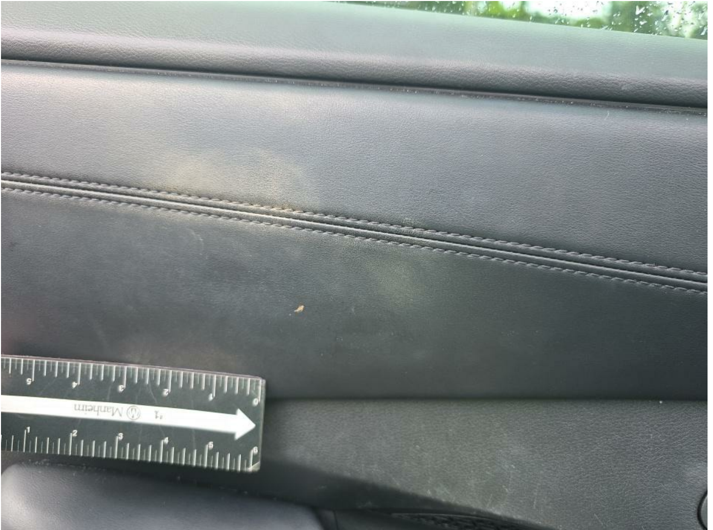
LF Door Panel Stained Permanent
