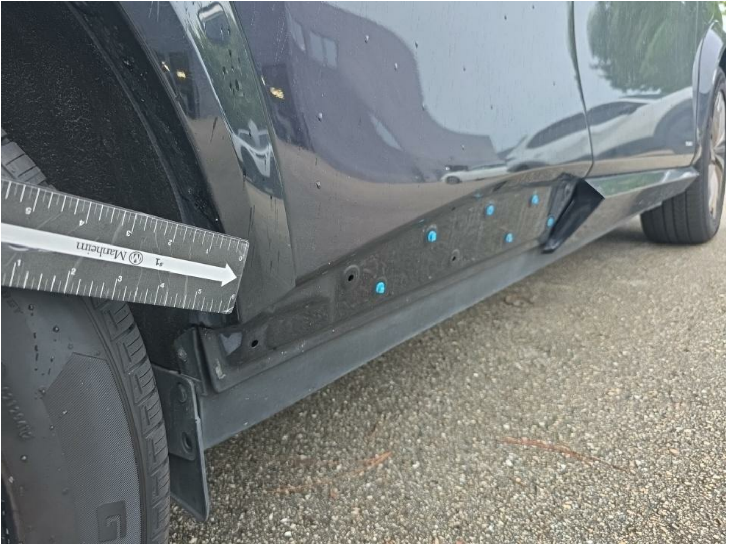
RR Door Molding Missing Replacement Required
