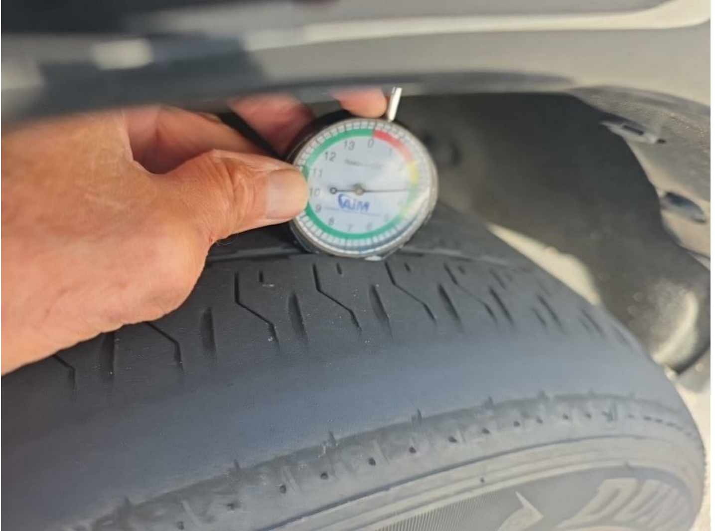
LR Tire Worn Replacement Required
