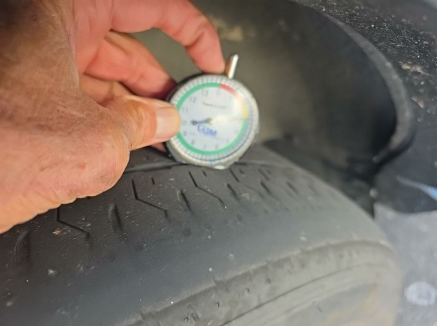
RR Tire Worn Replacement Required
