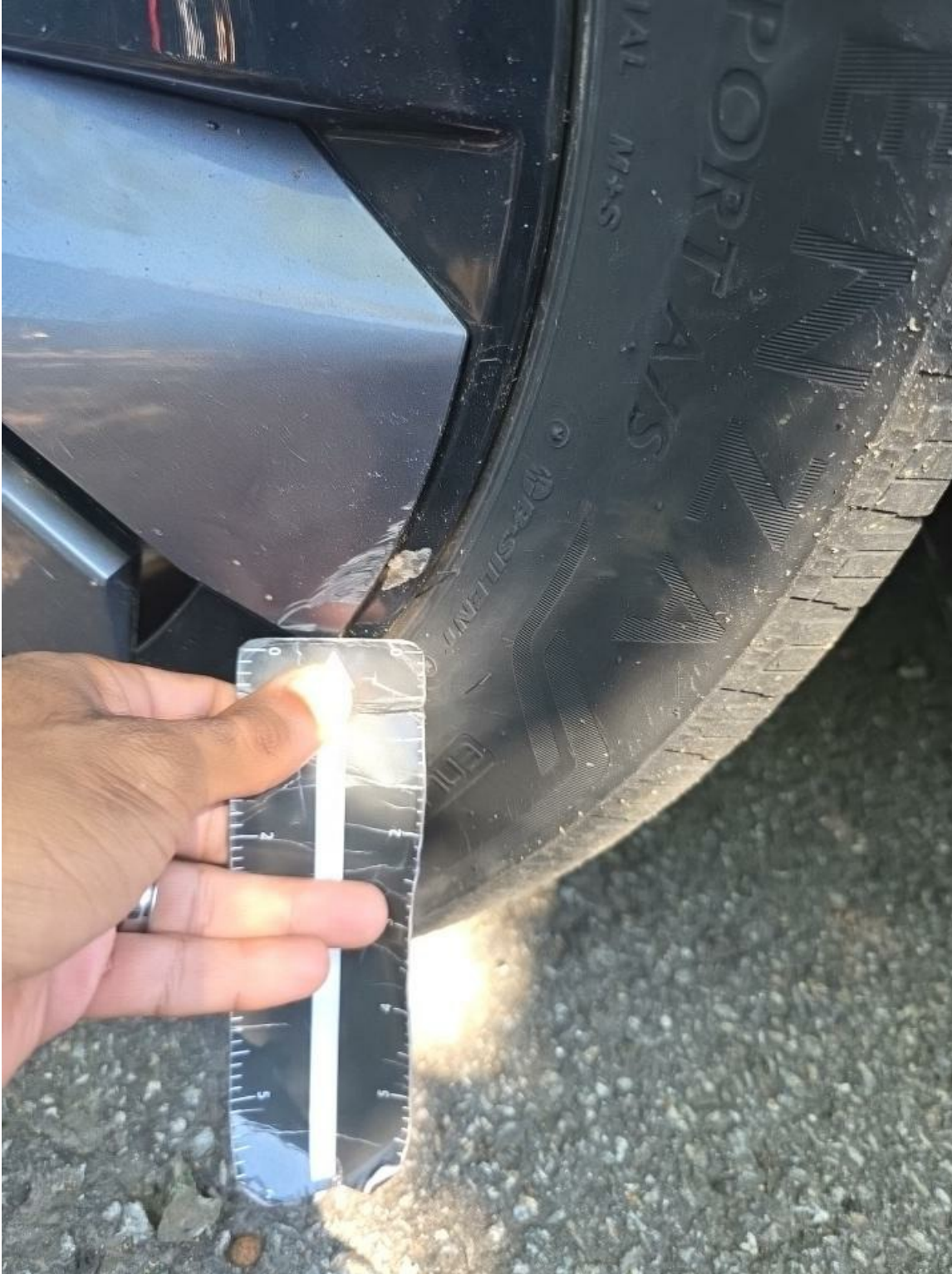
RR Wheel Curb Rash 1" to 2"
