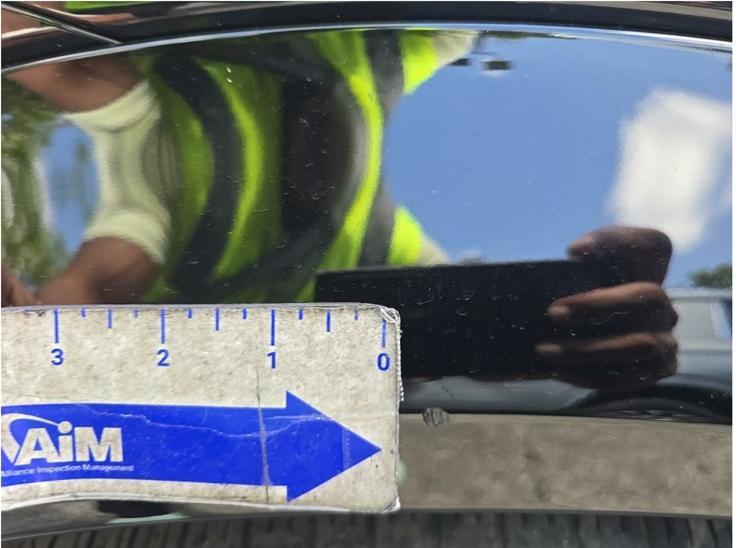
R Qtr Panel Molding Scratch Heavy 1" to 2"
