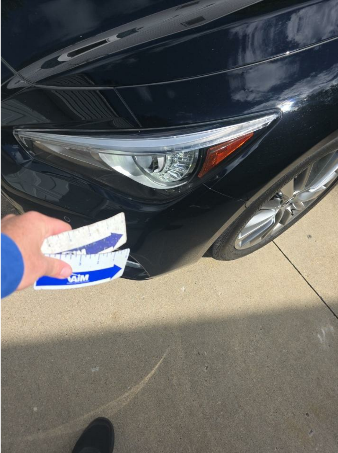
Front Bumper Cover Chipped 8
