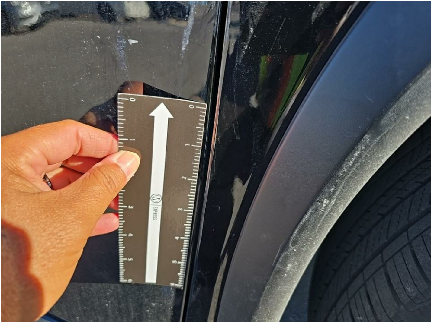
RF Fender Dent/Paint Dmg 1" to 2"
