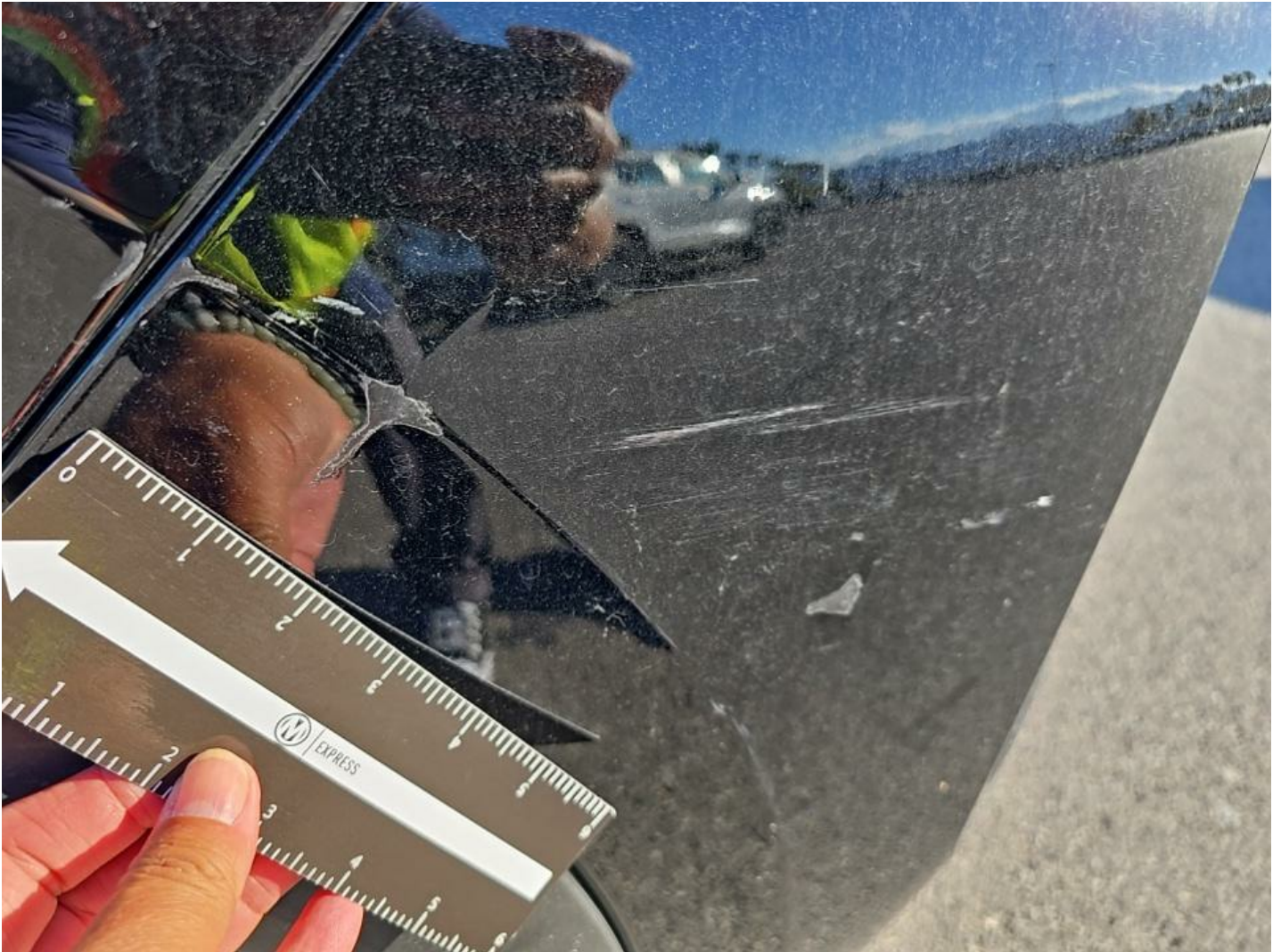
Front Bumper Cover Heavy Mult Scratches 5
