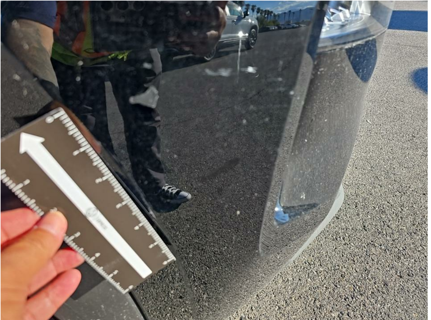
Front Bumper Cover Heavy Mult Scratches 5
