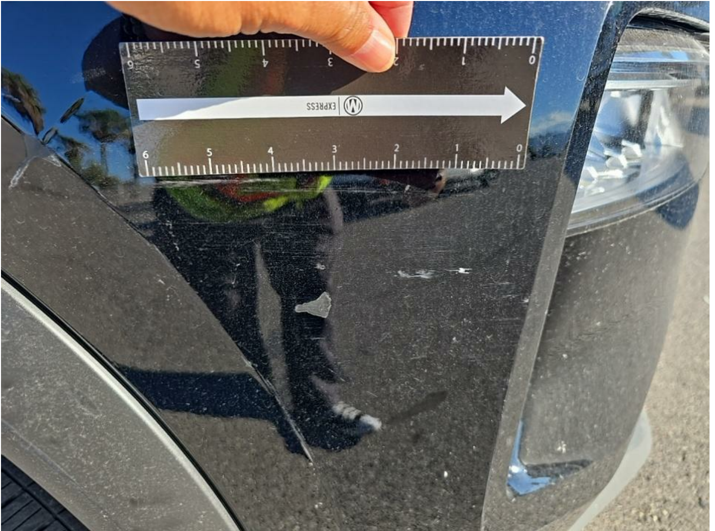
Front Bumper Cover Heavy Mult Scratches 5
