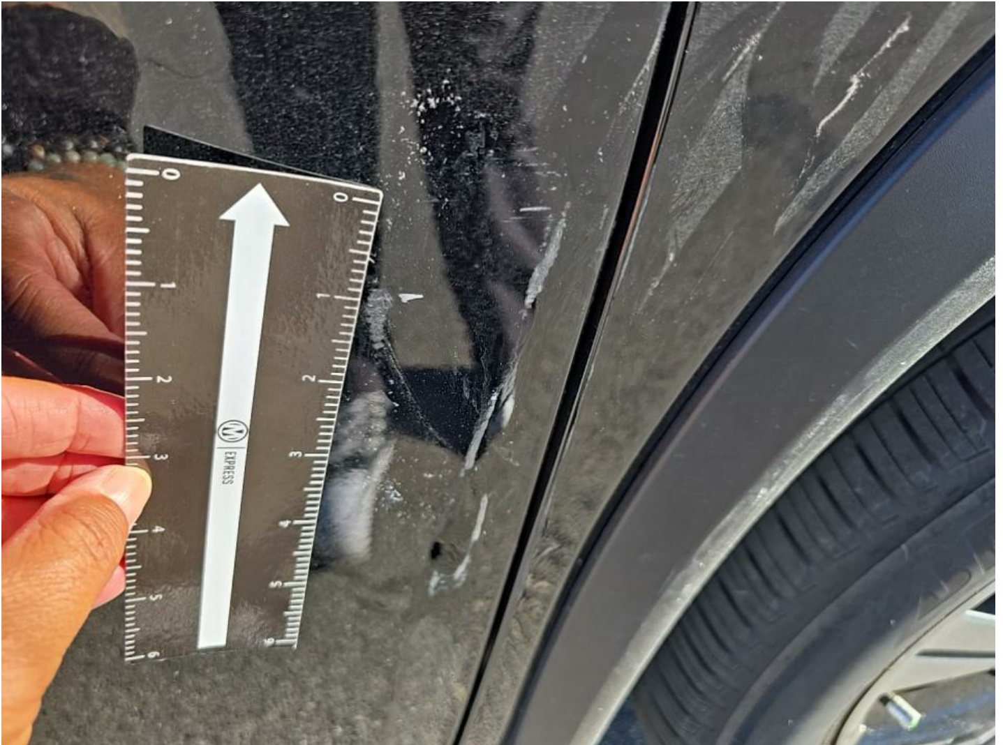
RF Door Dent/Paint Dmg 6" to 7"
