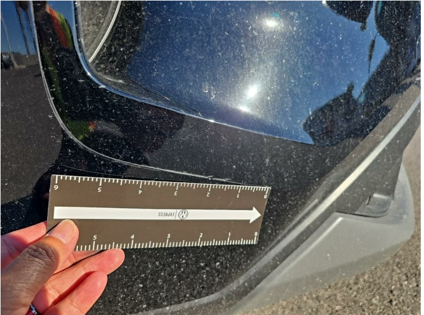
Front Bumper Cover Heavy Mult Scratches 5
