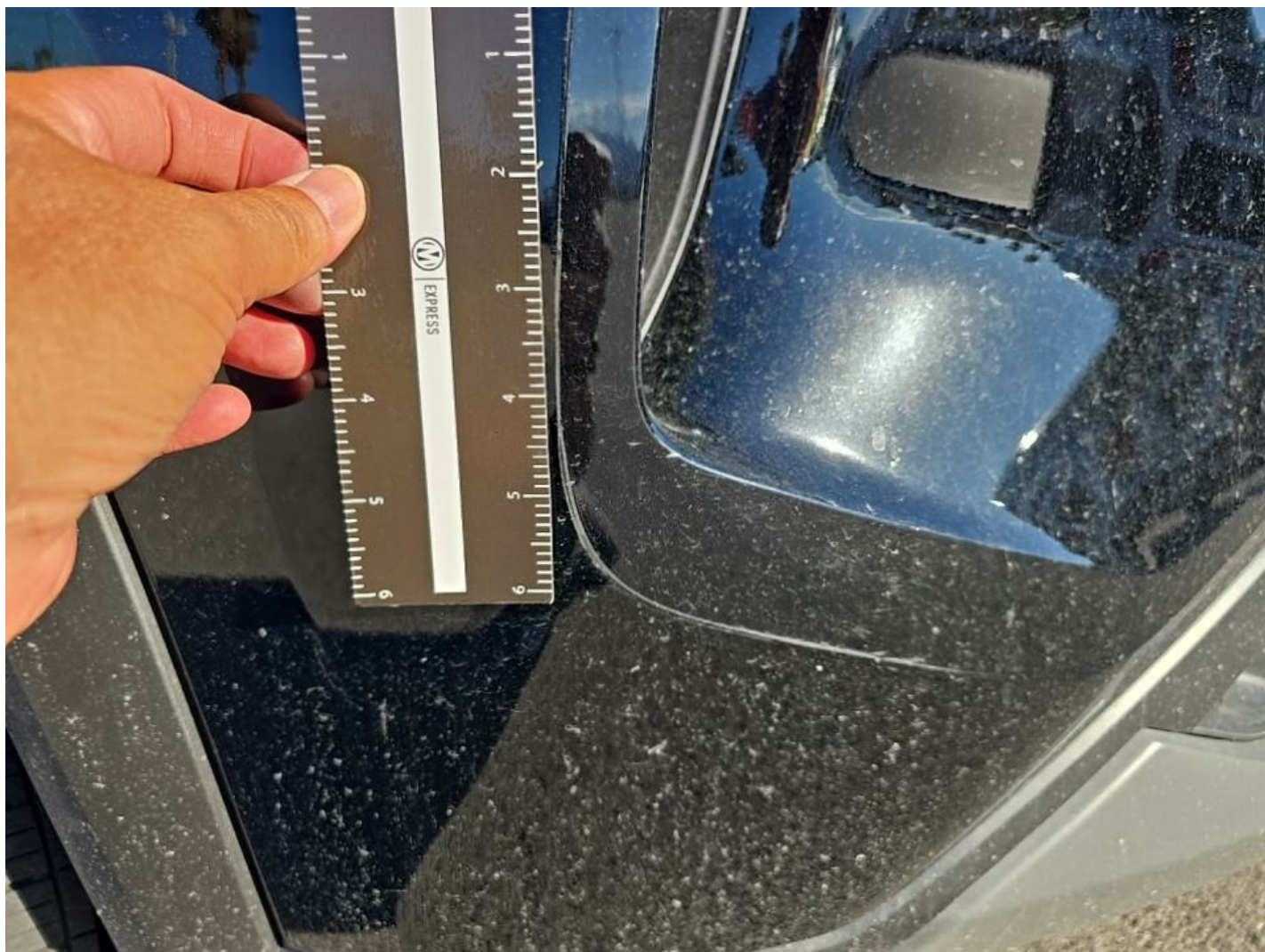
Front Bumper Cover Heavy Mult Scratches 5
