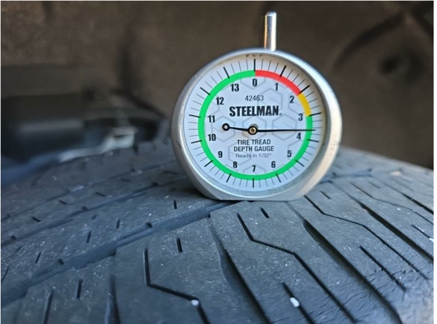
RR Tire Worn Replacement Required
