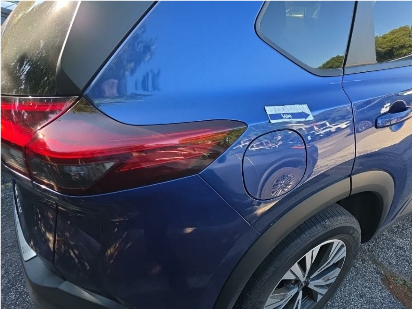
R Qtr Panel Prev Repair Acceptable
