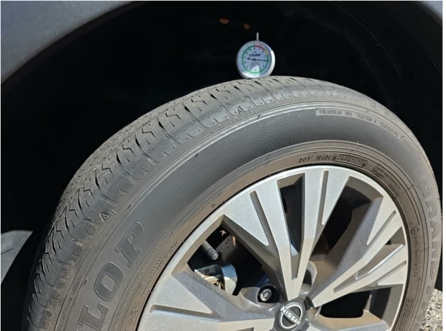
LF Tire Worn Replacement Required
