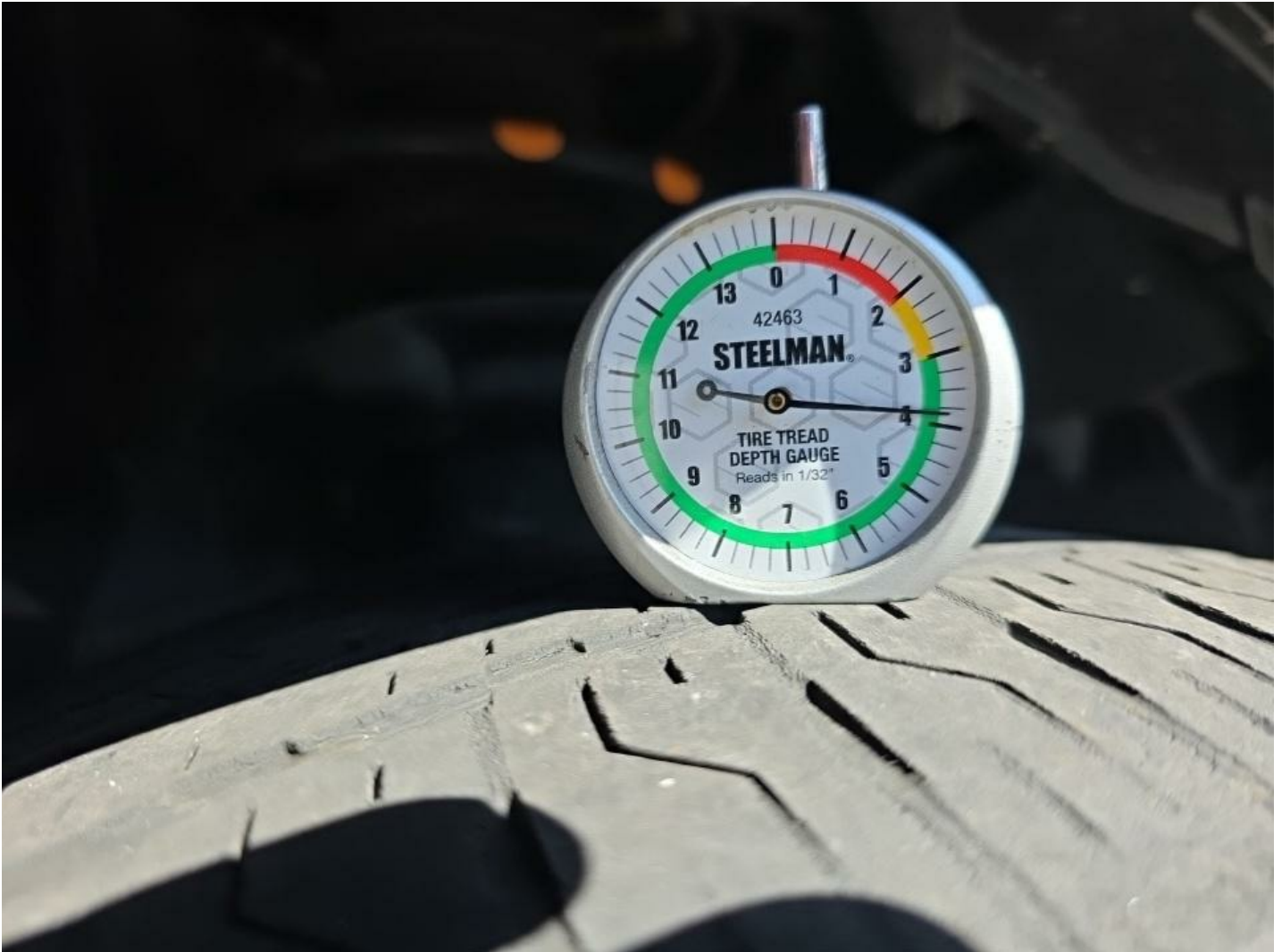
LF Tire Worn Replacement Required
