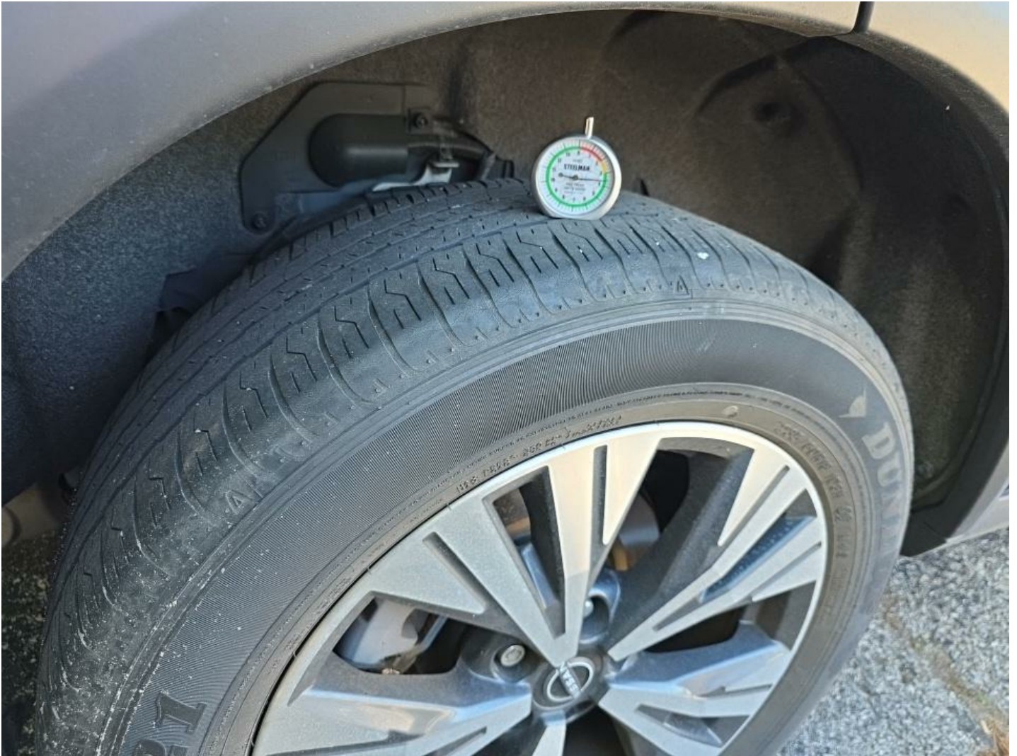
RR Tire Worn Replacement Required
