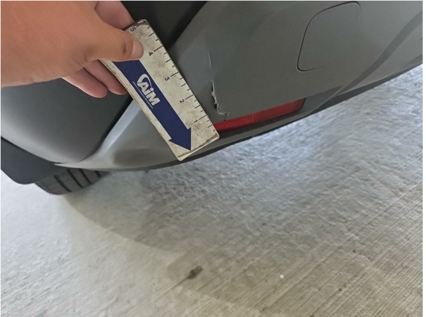
Rear Bumper Molding Cracked 1" to 2"
