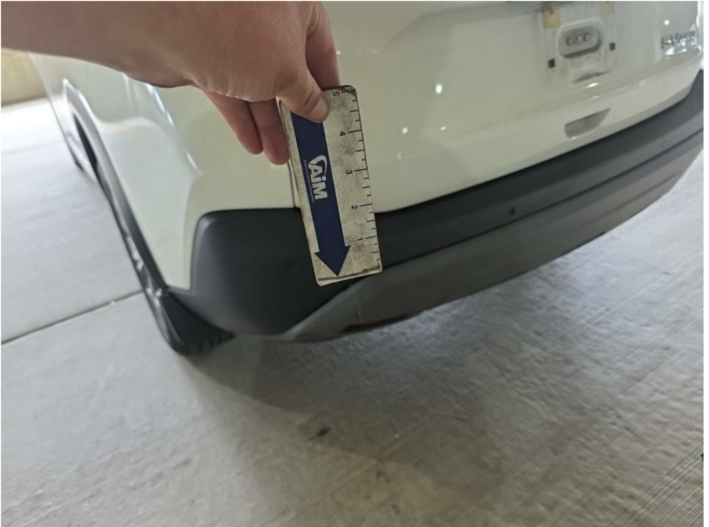
Rear Bumper Molding Cracked 1" to 2"
