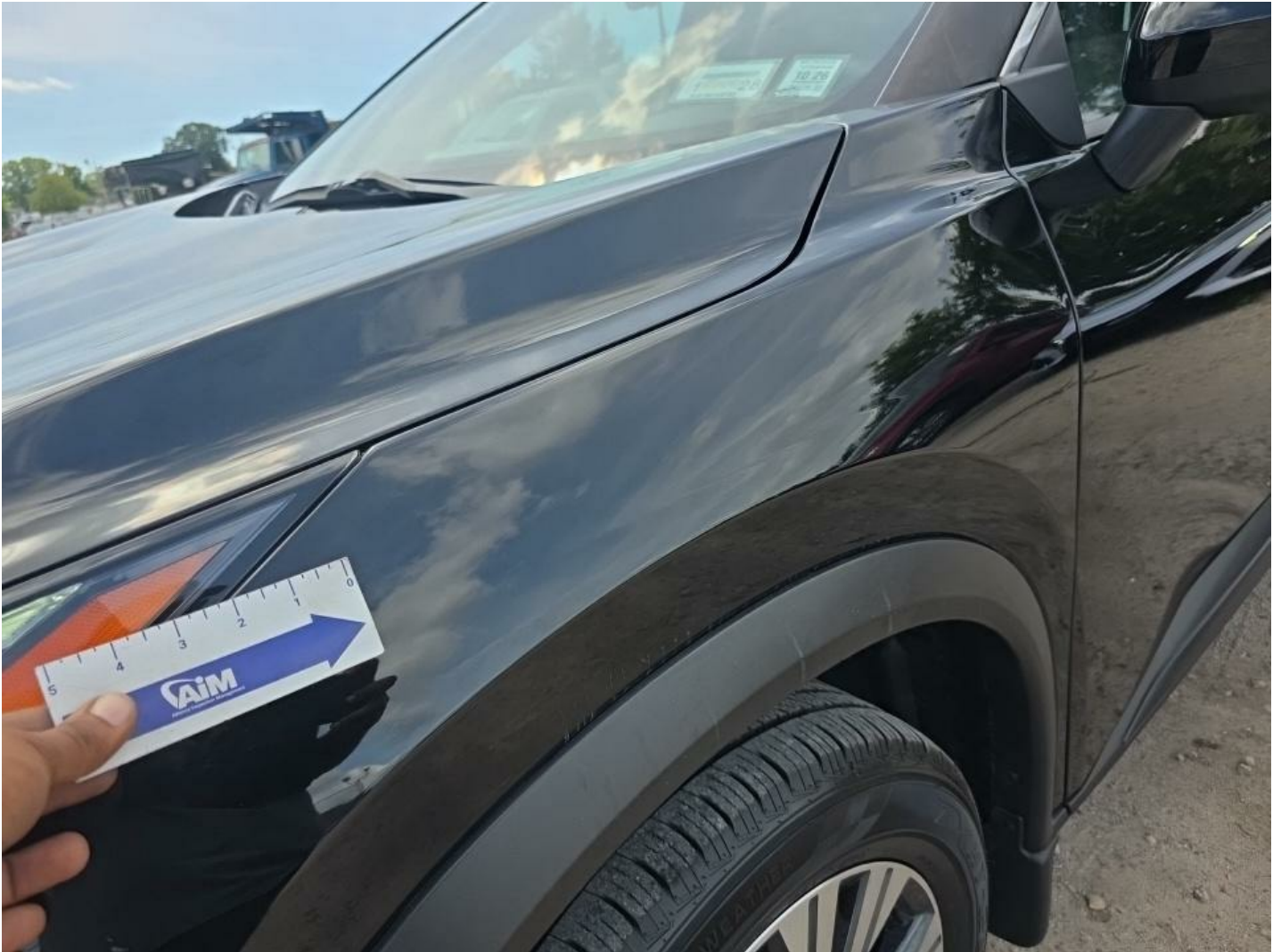
LF Fender Dent/No Paint Dmg GR 12"
