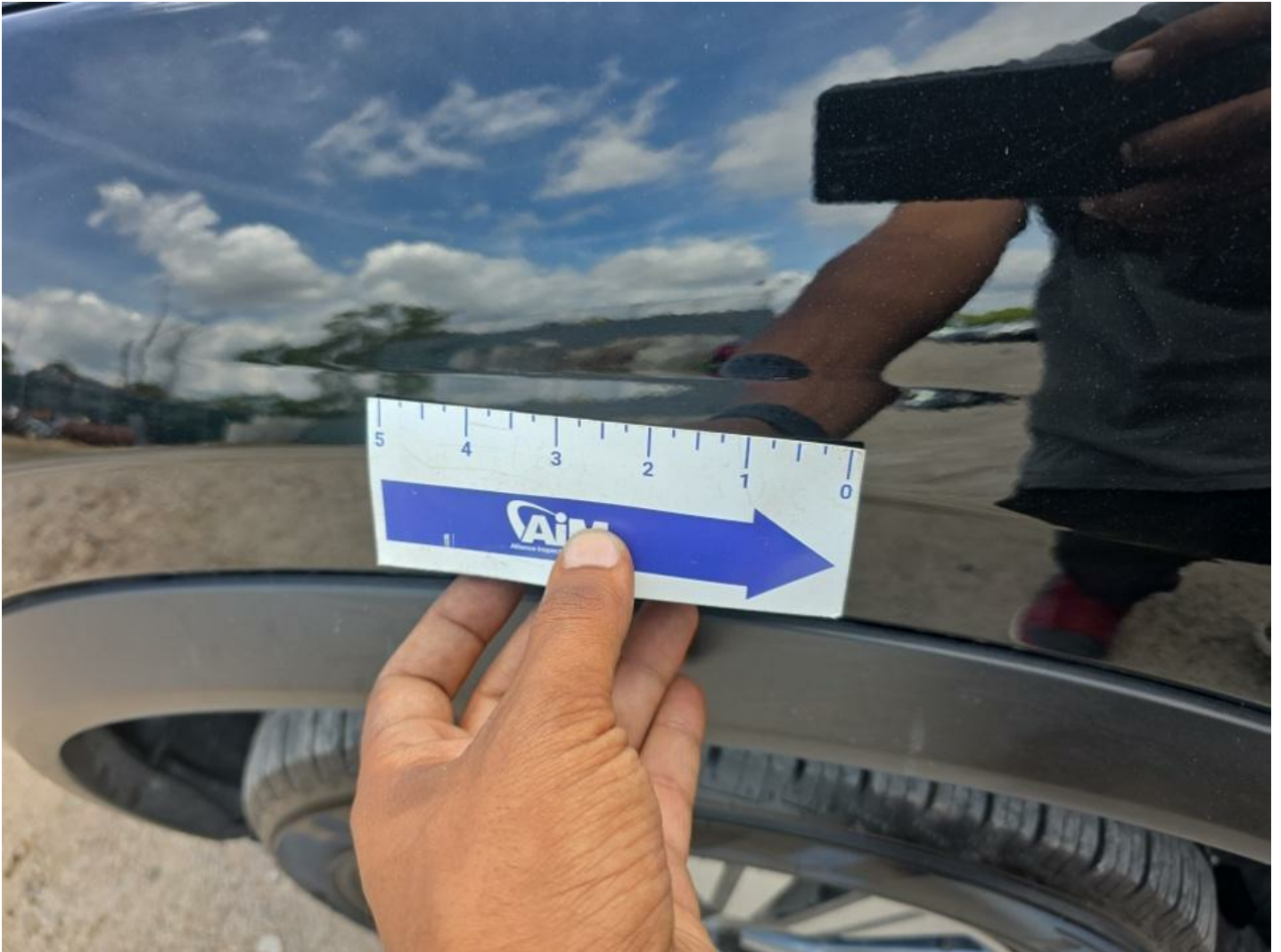
LF Fender Dent/No Paint Dmg GR 12"
