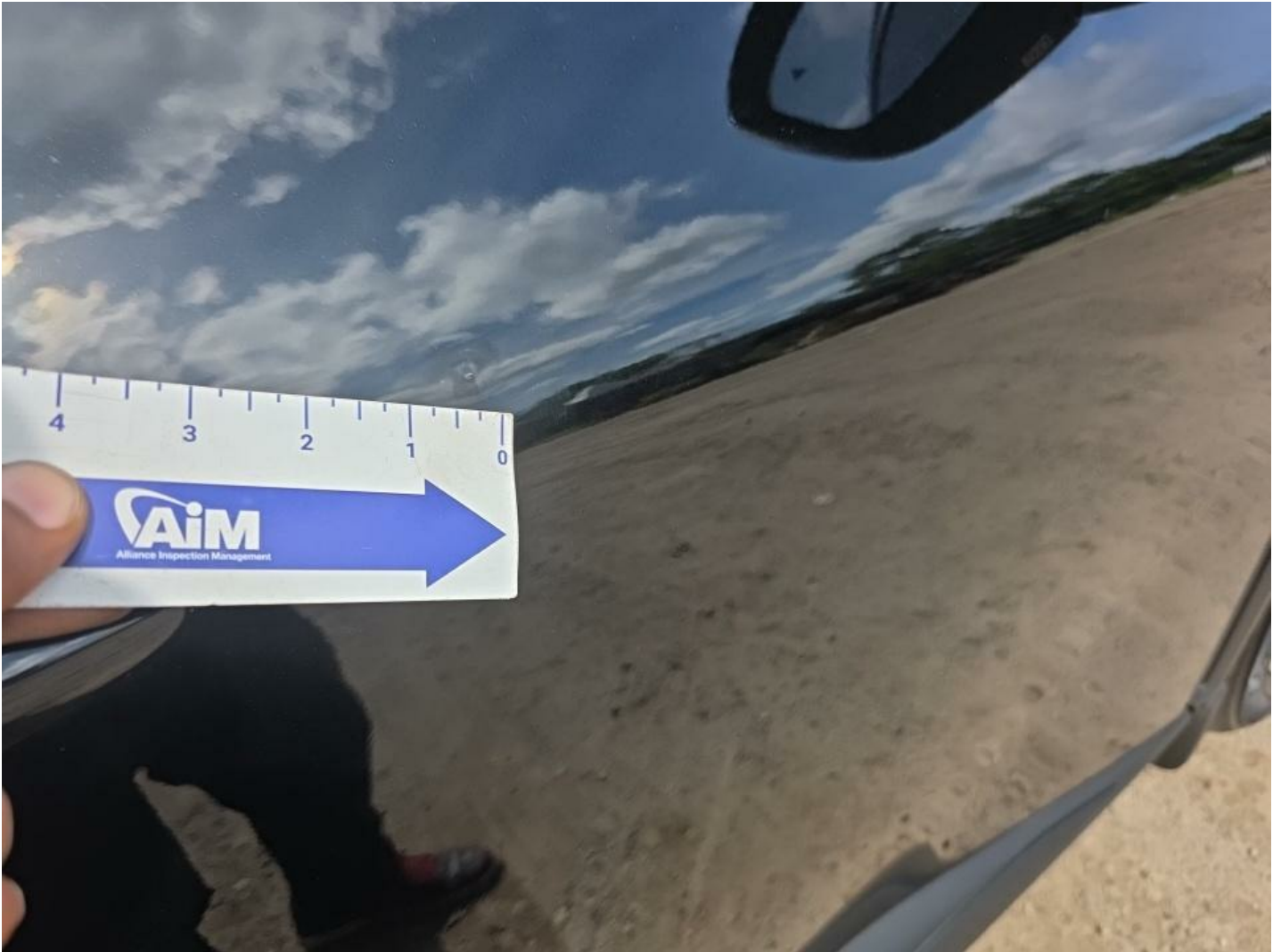
RF Door Dent/No Paint Dmg 1/2" to 1"
