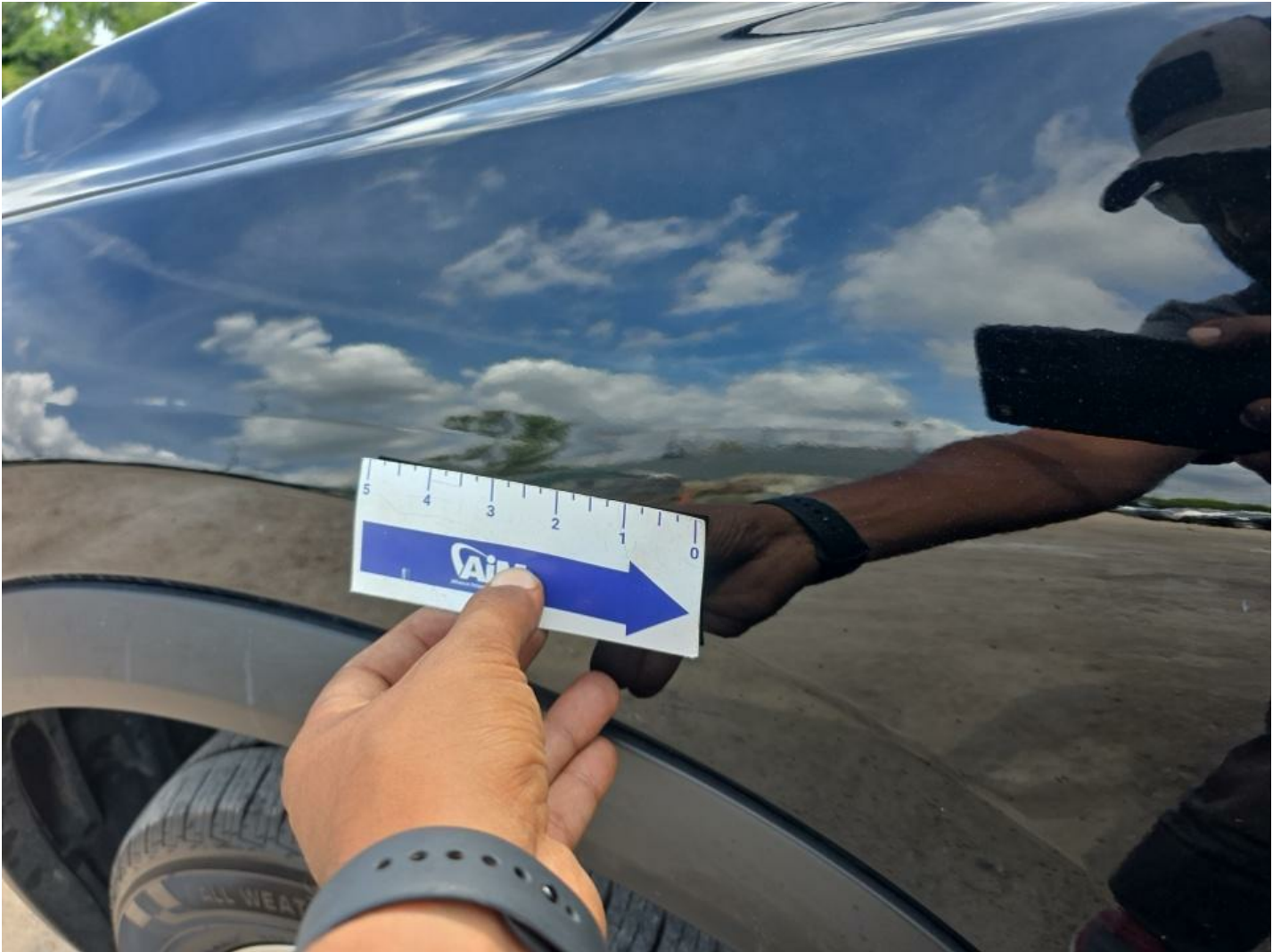
LF Fender Dent/No Paint Dmg GR 12"
