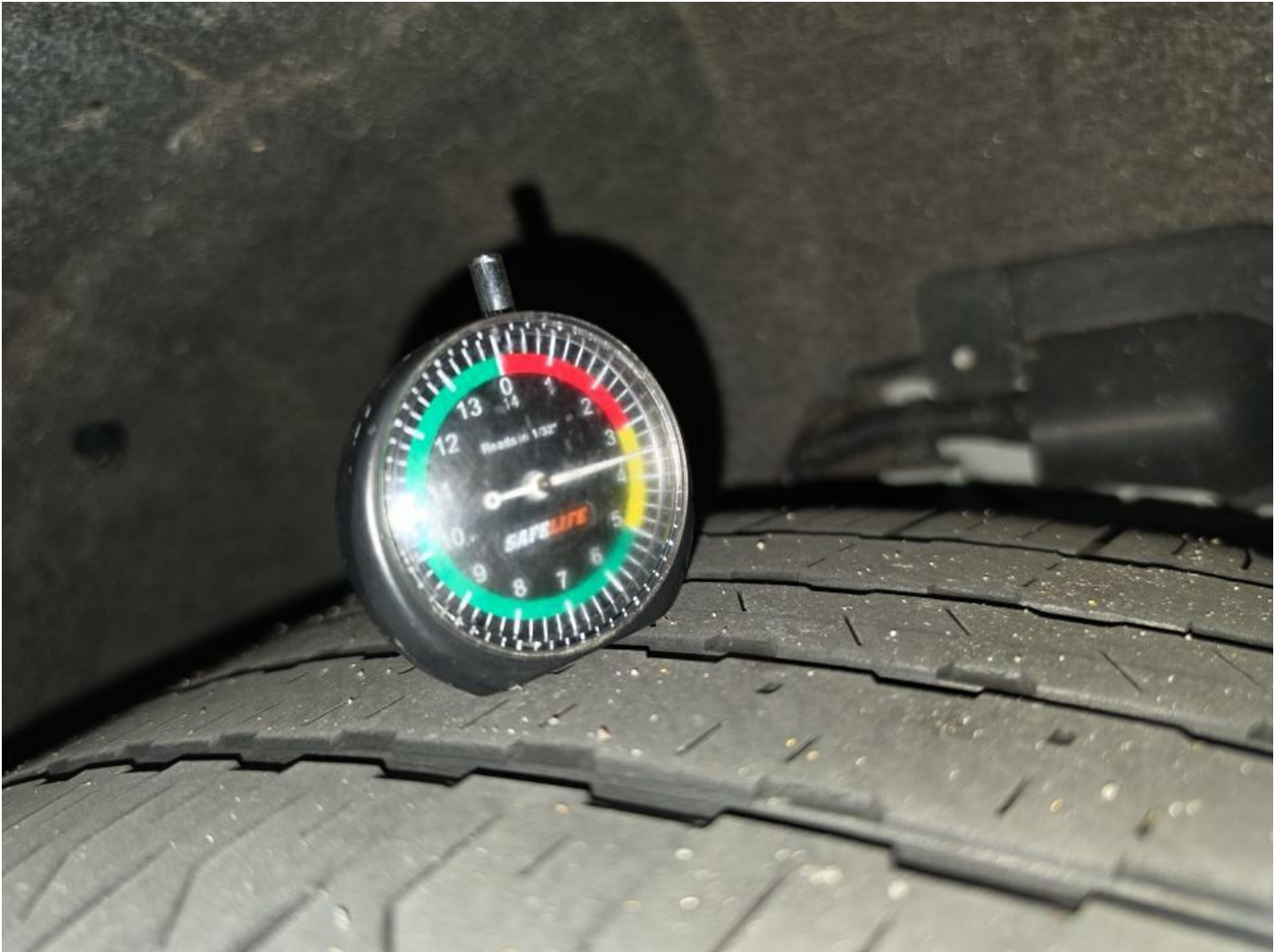
LR Tire Worn Replacement Required
