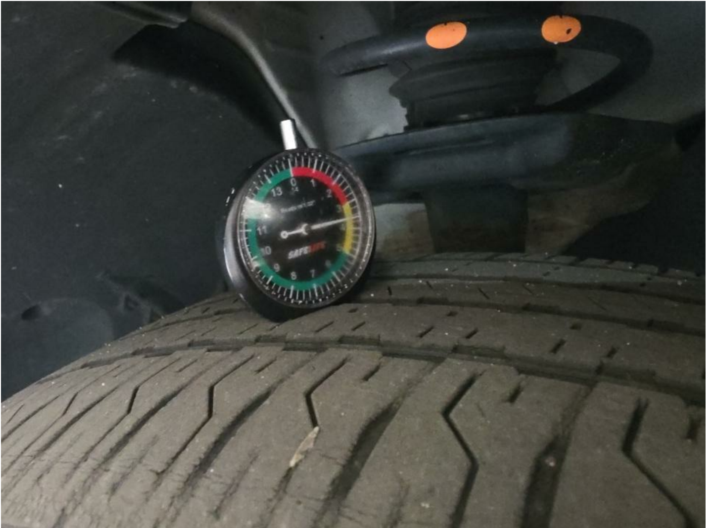
LF Tire Worn Replacement Required
