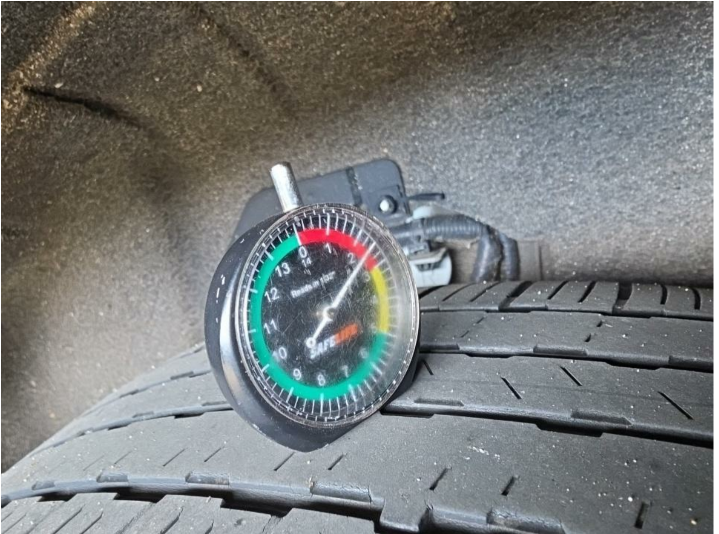
RR Tire Worn Replacement Required
