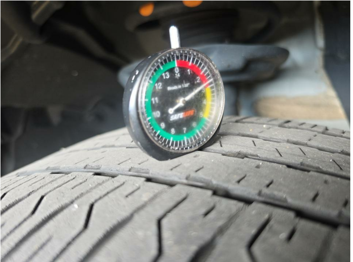
RF Tire Worn Replacement Required
